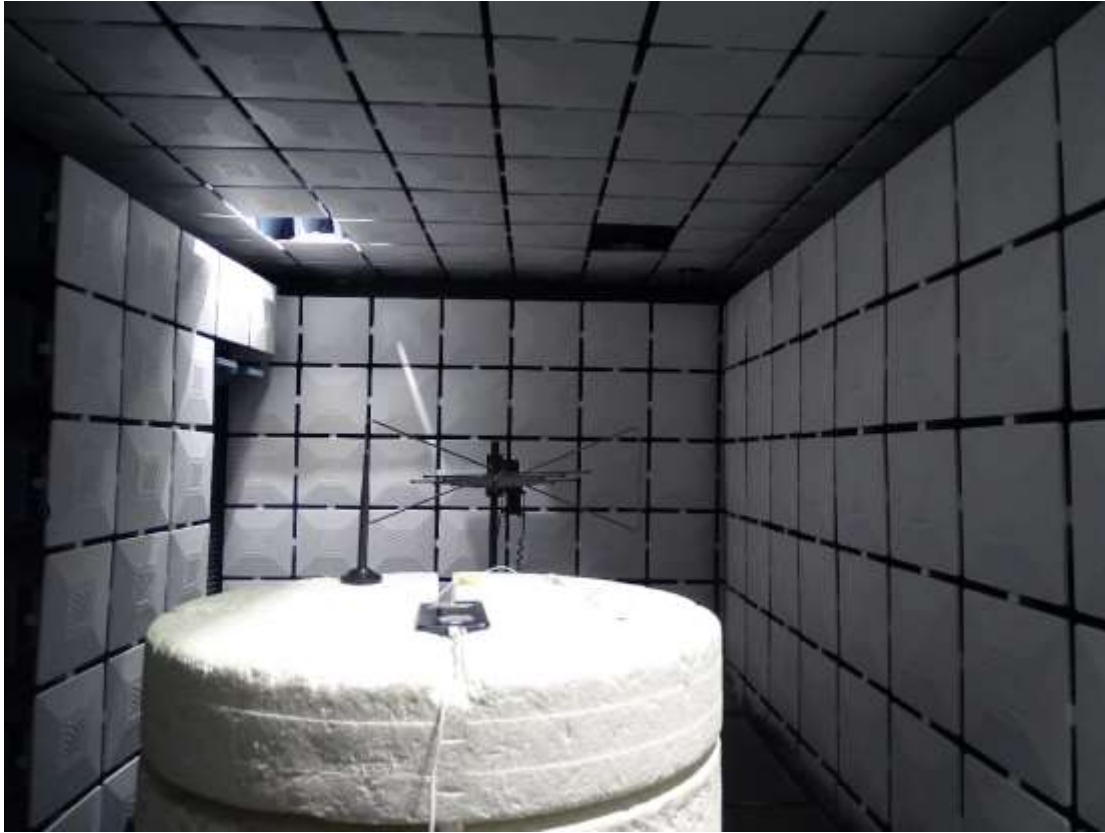
Radiated Spurious Emission (30MHz to 3GHz)
