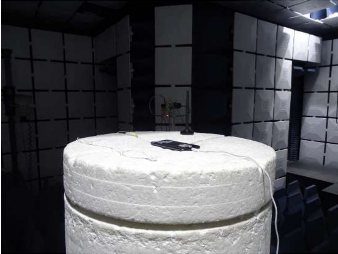
Radiated Spurious Emission (18GHz to26.5GHz)
