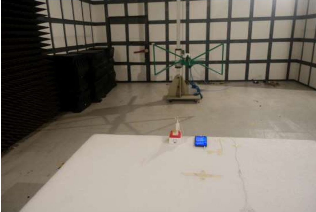
Radiated Spurious Emission (30MHz to 1GHz)
