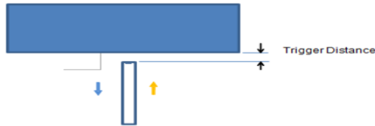
Picture: Proximity sensor triggering distances assessment (Bottom side)
