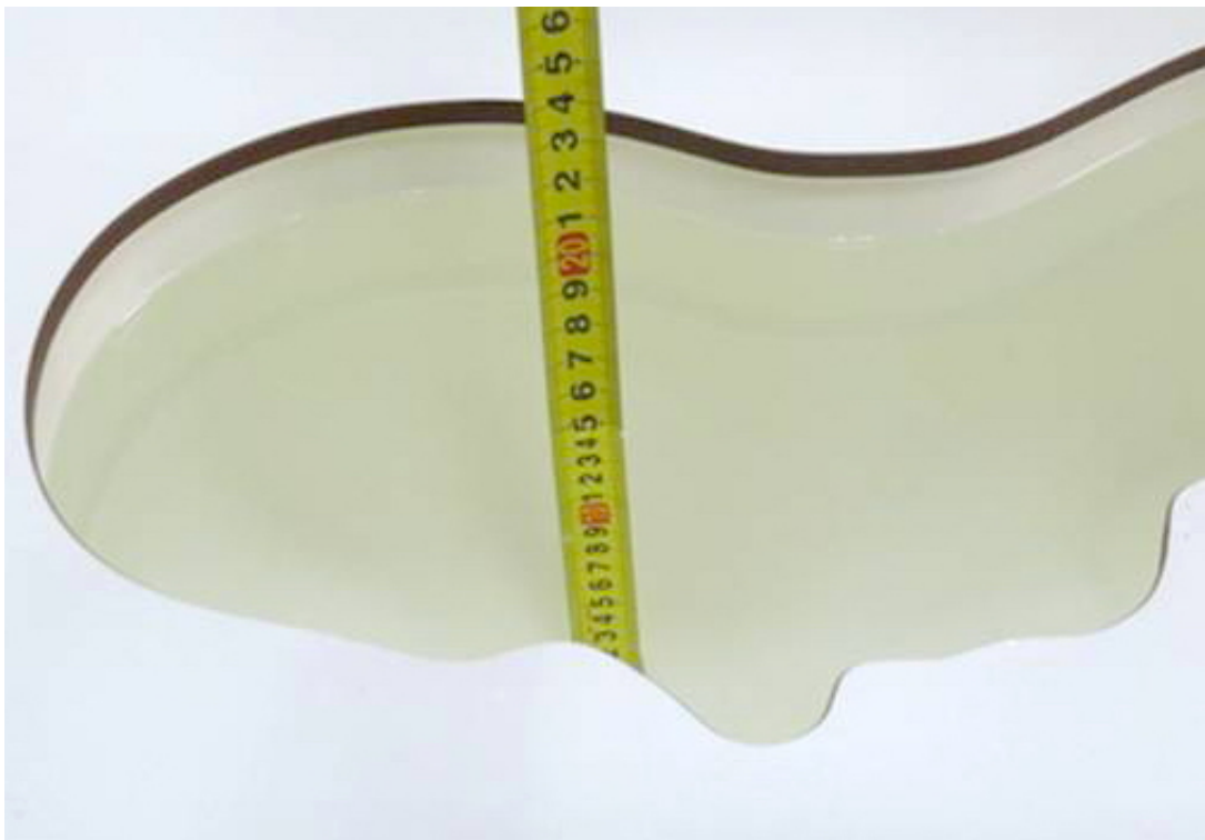
Picture 13: Liquid depth in the head Phantom (5800 MHz, 15.4cm depth)
