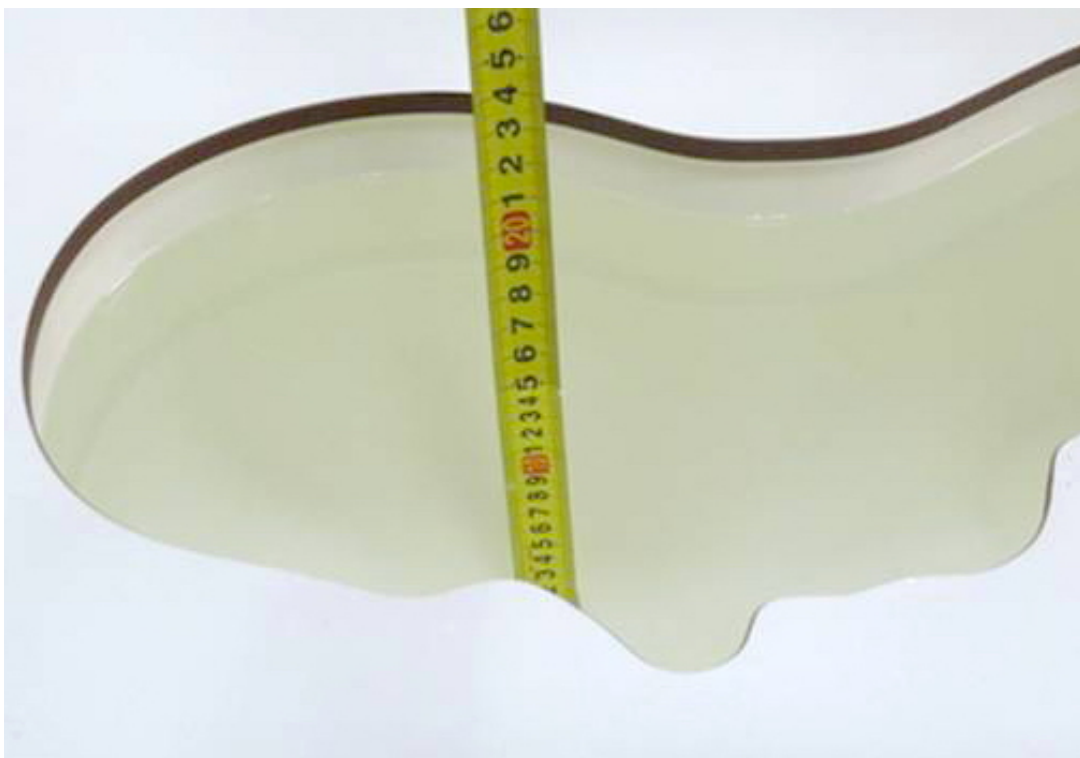
Picture 11: Liquid depth in the head Phantom (5600 MHz, 15.4cm depth)
