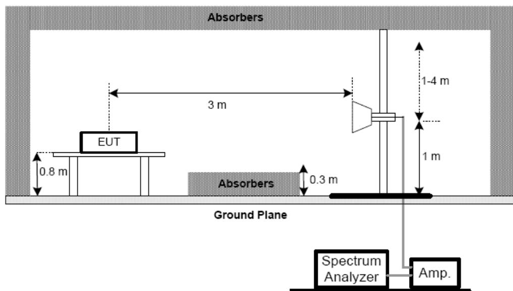
(C) For radiated emissions below 30MHz
