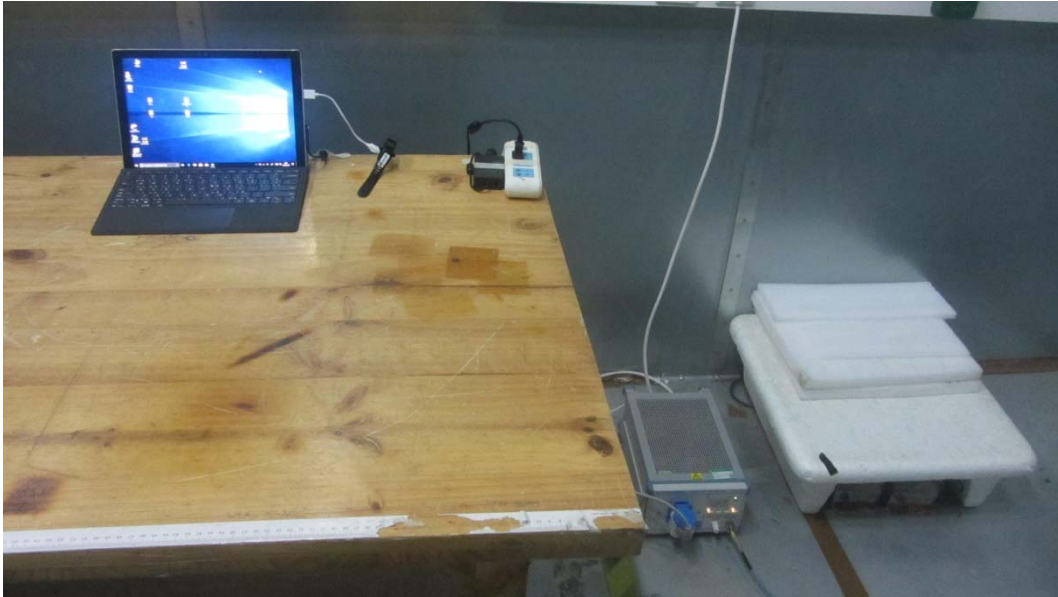
Picture 2 Conducted Emission Test Setup
