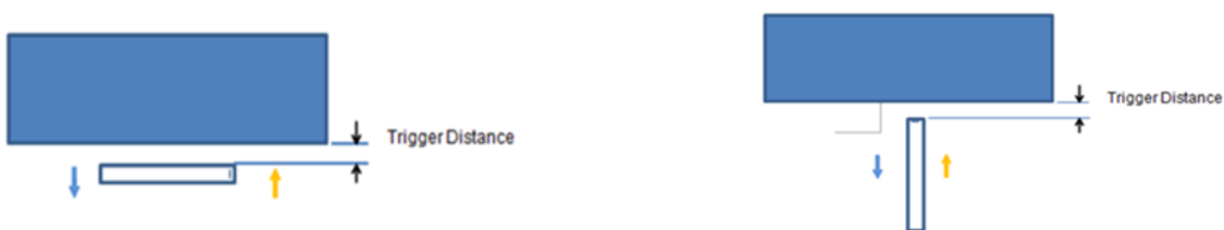
Picture: Proximity sensor triggering distances assesment for the back side Picture: Proximity sensor triggering distances assesment for the Top side
