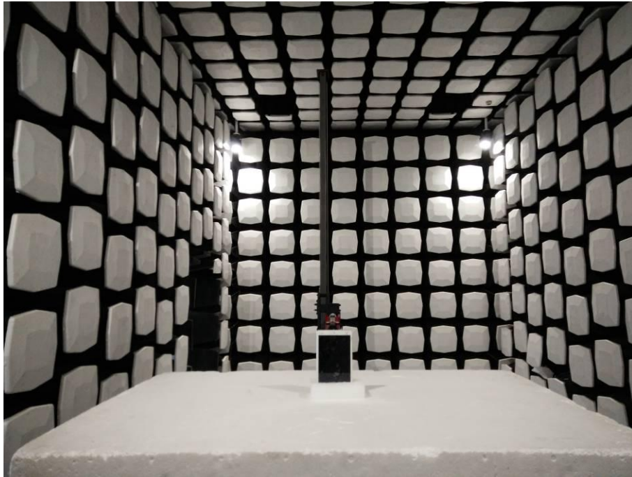
7. Radiated Emissions (Part 15C) (1-18GHz)
