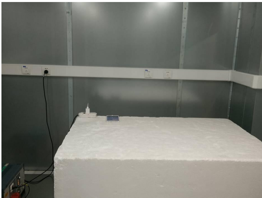
10. Conducted Emission (Part 15B Charging mode)
