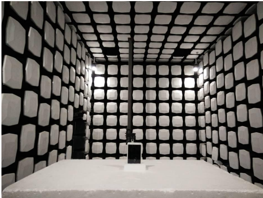
8. Radiated Emissions (Part 15C) (18-26.5GHz)
