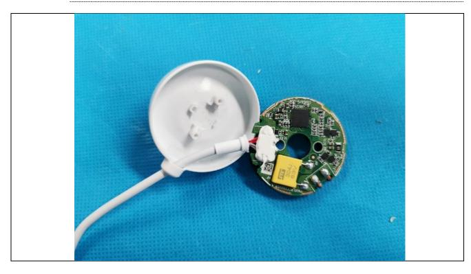
Details of: PCB and coil view 2
