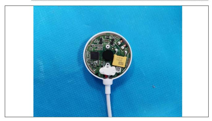
Details of: PCB and coil view 1
