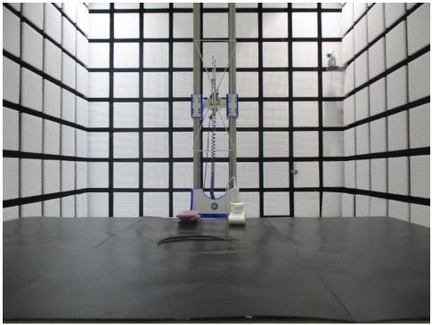
Radiated Disturbance Emissions (30MHz-1GHz)
