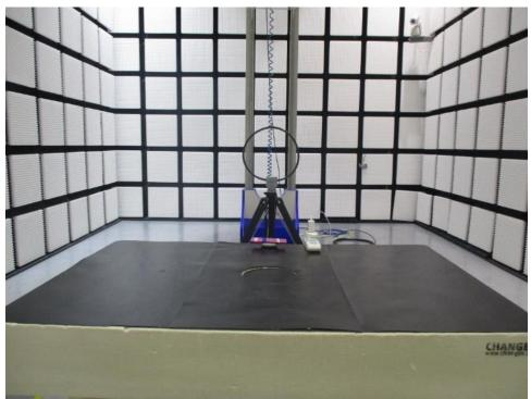
Radiated Disturbance Emissions (9kHz-30MHz)
