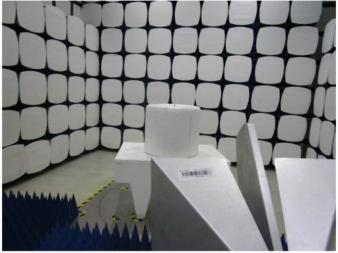
1.2 Radiated Spurious Emissions Test Setup
