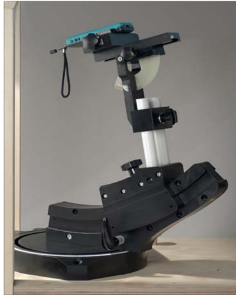
F-2. Device Holder for Transmitters
