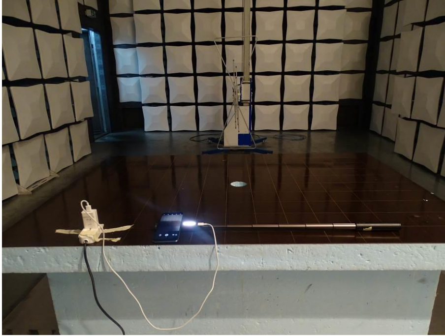
Radiated Disturbance Emissions (below 1GHz)
