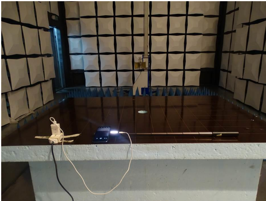
Radiated Disturbance Emissions (1GHz to18GHz)
