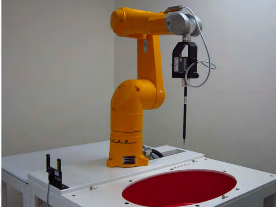
Fig.1 Photograph of the SAR measurement system
