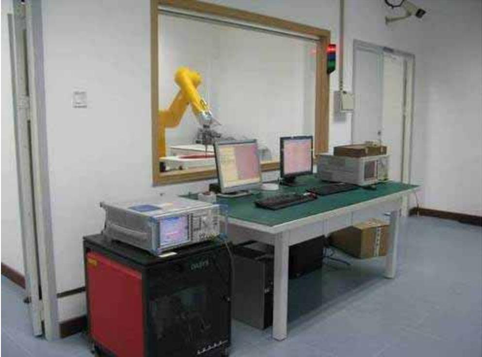
Photo 2: Measurement System DASY5
