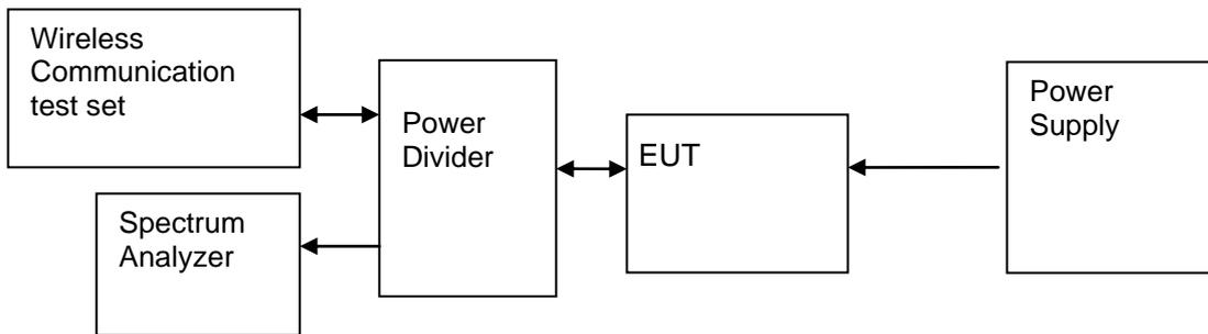
Figure 2. Test Set-up
