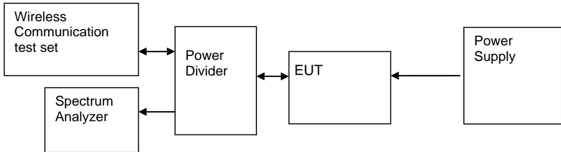
Figure 3. Test Set-up
