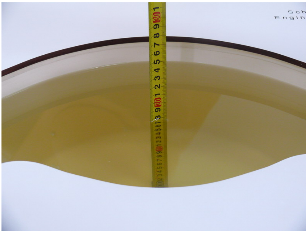
Picture 2: Liquid depth in the Flat Phantom (835 MHz)
