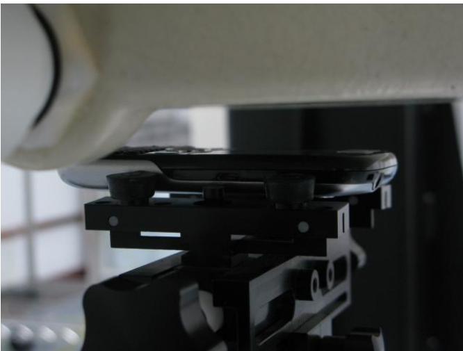
Photo 11: HUAWEI M635 body worn rear side with Headset (15mm distance)
