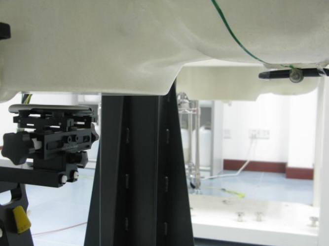
Photo 12: HUAWEI M635 body worn rear side with Bluetooth Headset (15mm distance)
