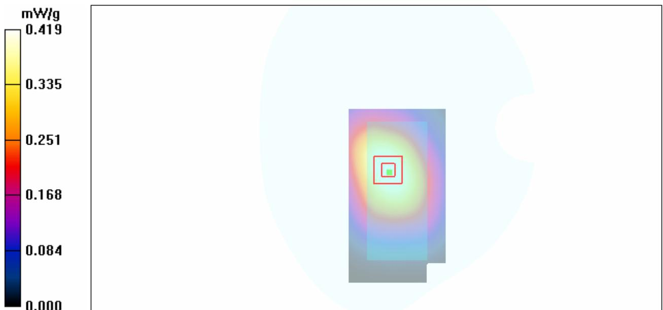
Figure 18 Body, Towards Phantom, CDMA Cellular Channel 384
