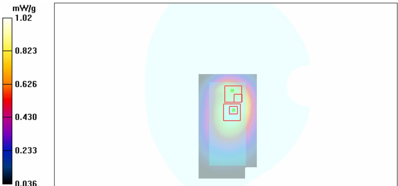
Figure 16 Body, Towards Ground, CDMA Cellular Channel 384
