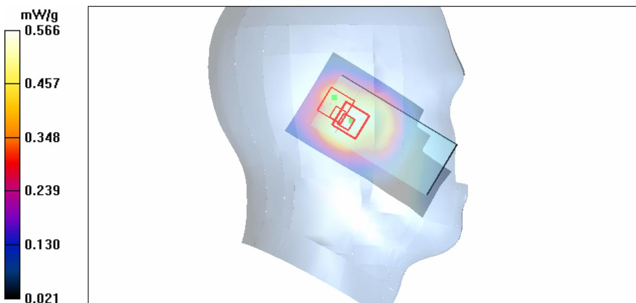
Figure 9 Left Hand Touch Cheek CDMA Cellular Channel 384
