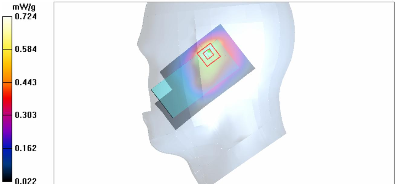
Figure 12 Right Hand Touch Cheek CDMA Cellular Channel 384
