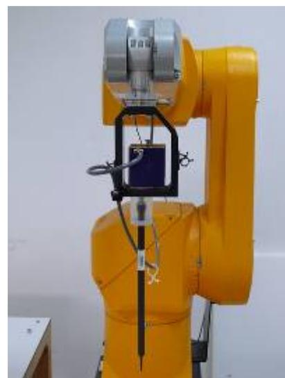
Figure 3. EX3DV4 E-field probe
