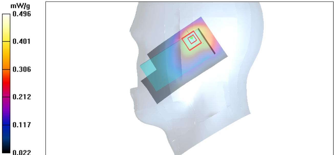
Figure 14 Right Hand Tilt 15° CDMA Cellular Channel 384
