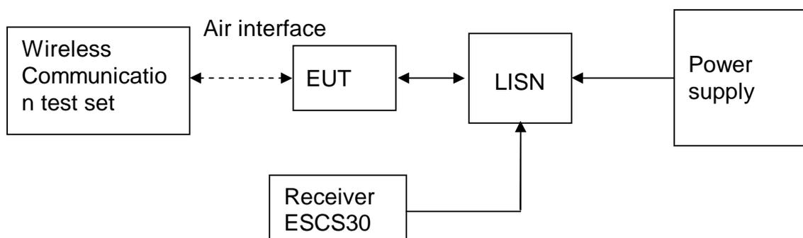
Figure 3. Test Set-up
