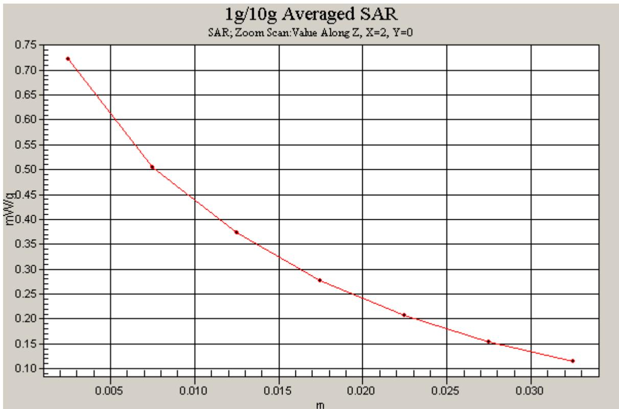
Figure 14 Z-Scan at power reference point (Left Hand Touch Cheek CDMA Cellular Channel 1013)
