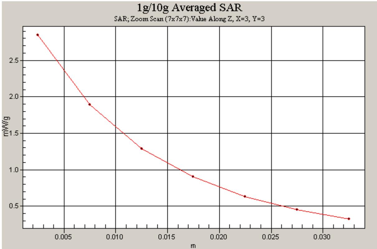
Figure 8 Z-Scan at power reference point (system Check at 835 MHz dipole)
