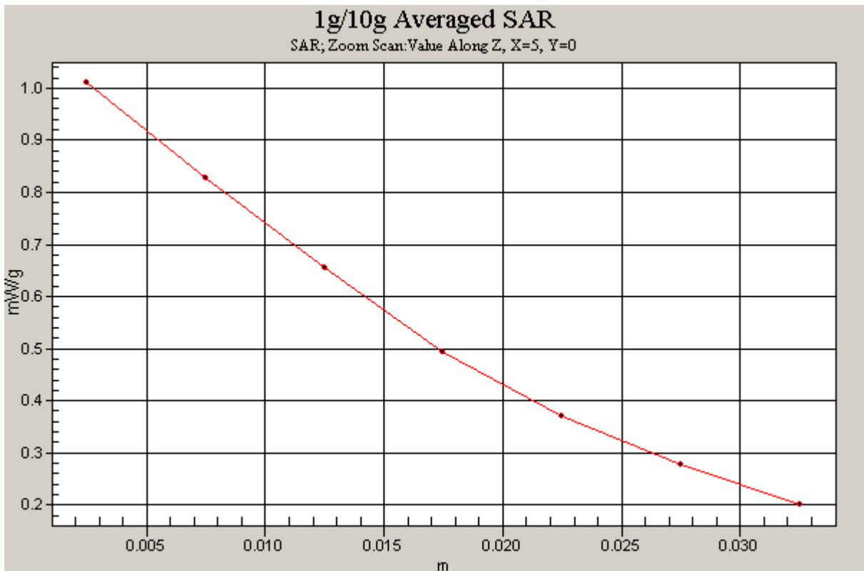
Figure 10 Z-Scan at power reference point (Left Hand Touch Cheek CDMA Cellular Channel 777)
