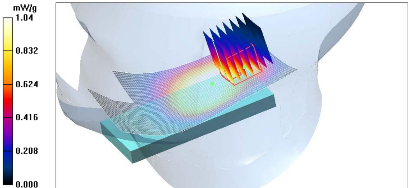
Figure 21 Right Hand Touch Cheek CDMA Cellular Channel 777
