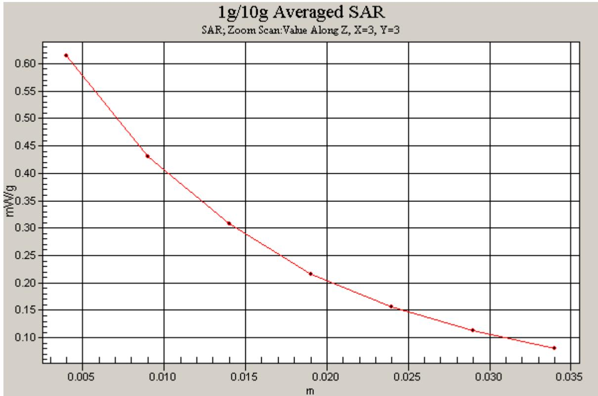
Figure 46 Z-Scan at power reference point (Body with earphone, Towards Ground, , CDMA Cellular Channel 1013)
