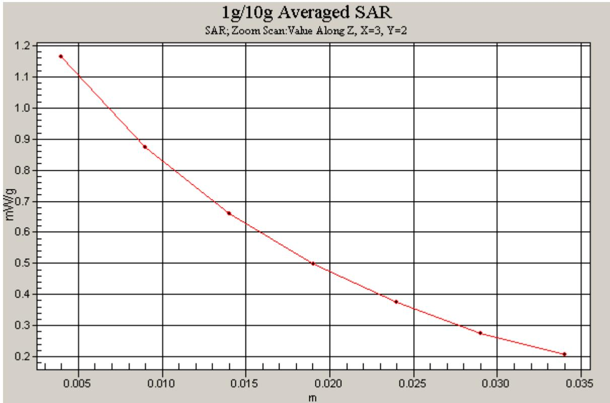
Figure 48 Z-Scan at power reference point (Body with Bluetooth earphone, Towards Ground, , CDMA Cellular Channel 1013)
