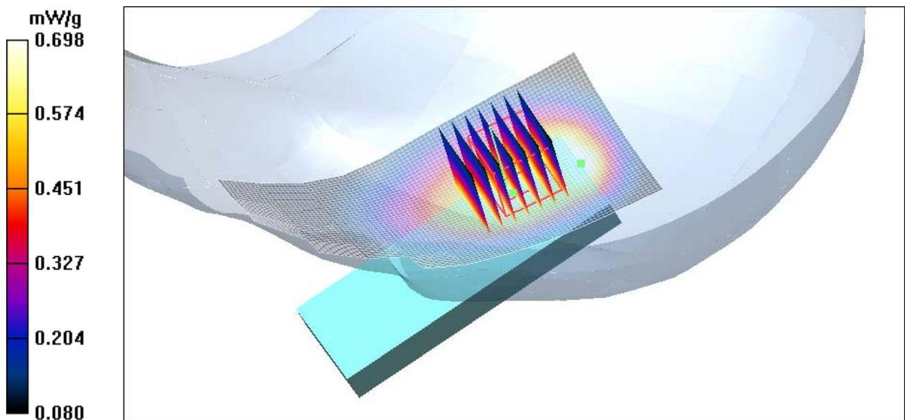
Figure 15 Left Hand Tilt 15°CDMA Cellular Channel 777
