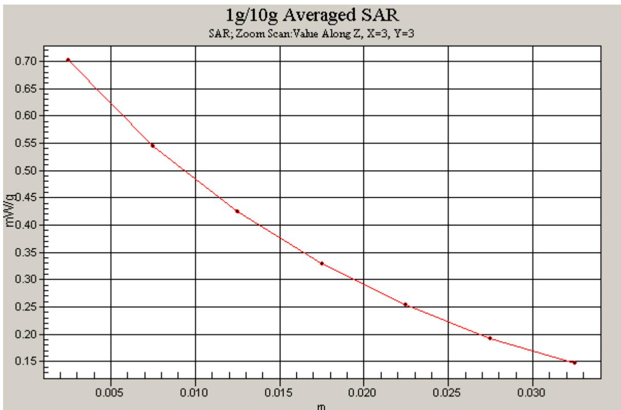
Figure 30 Z-Scan at power reference point (Right Hand Tilt 15°CDMA Cellular Channel 384)
