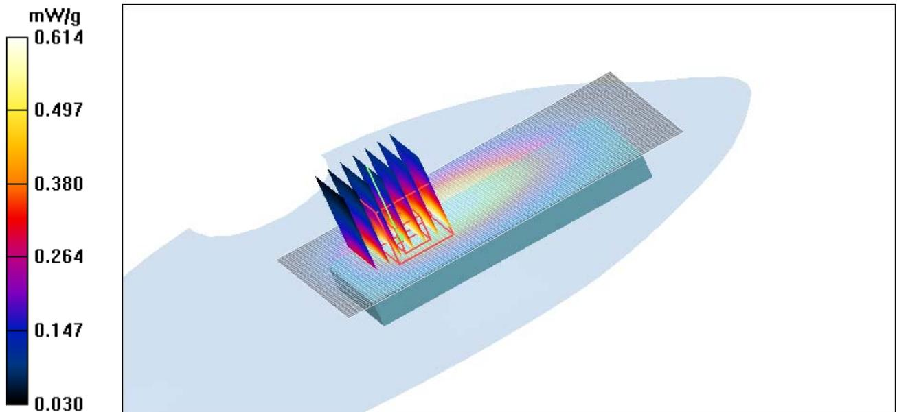
Figure 45 Body with earphone, Towards Ground, CDMA Cellular Channel 1013
