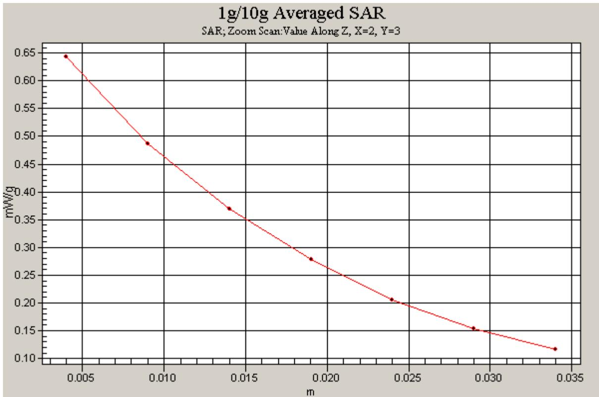
Figure 40 Z-Scan at power reference point (Body, Towards Phantom, , CDMA Cellular Channel 777)
