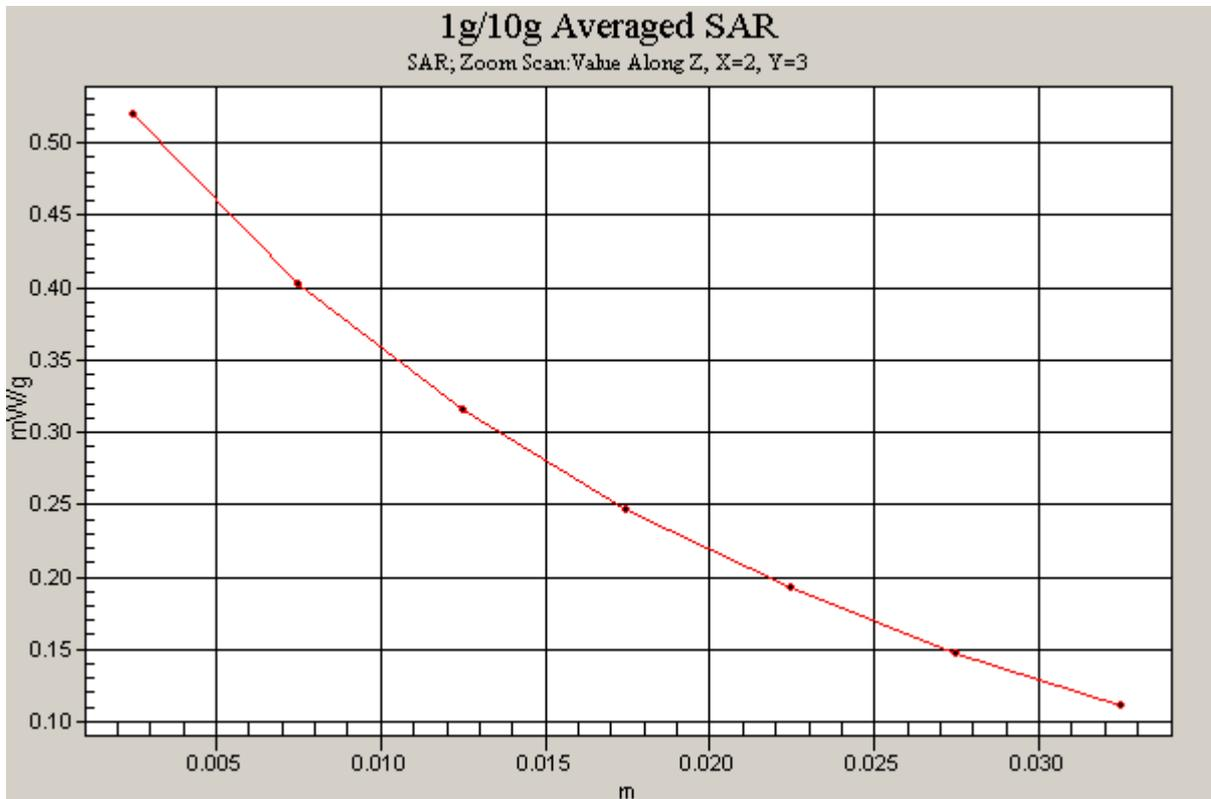
Figure 20 Z-Scan at power reference point (Left Hand Tilt 15°CDMA Cellular Channel 1013)
