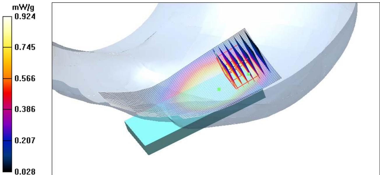
Figure 11 Left Hand Touch Cheek CDMA Cellular Channel 384
