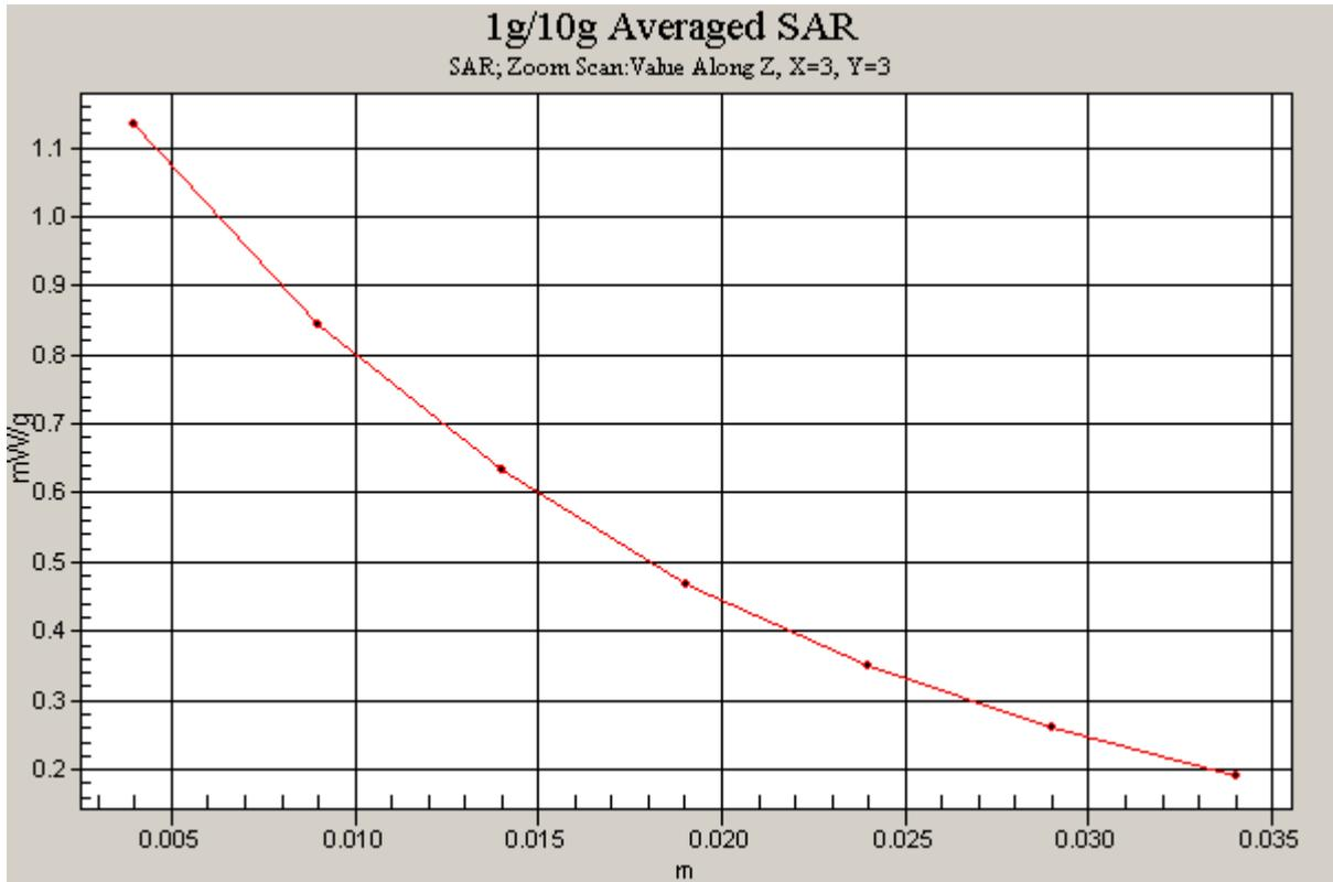
Figure 34 Z-Scan at power reference point (Body, Towards Ground, CDMA Cellular Channel 777)
