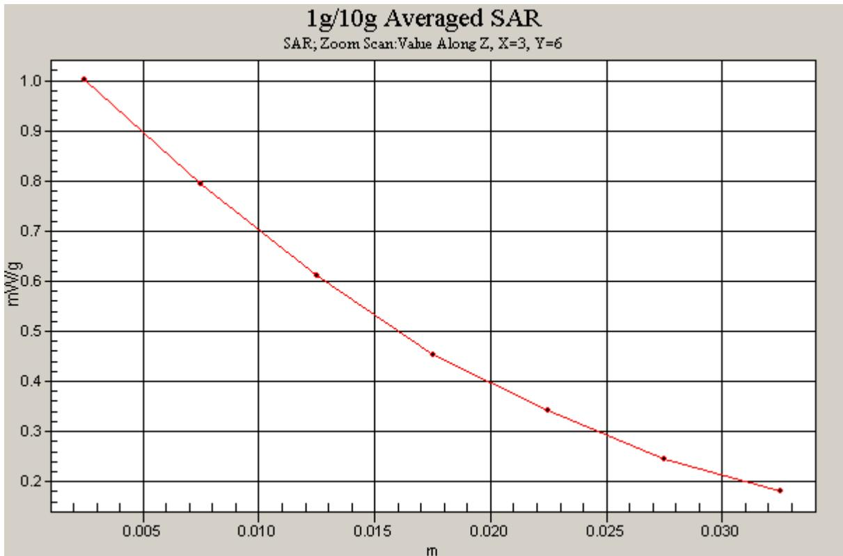
Figure 24 Z-Scan at power reference point (Right Hand Touch Cheek CDMA Cellular Channel 384)
