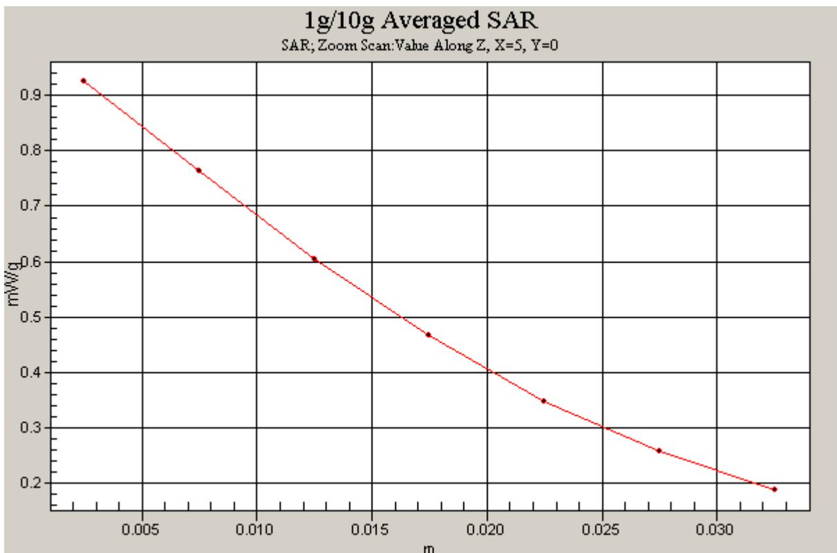
Figure 12 Z-Scan at power reference point (Left Hand Touch Cheek CDMA Cellular Channel 384)
