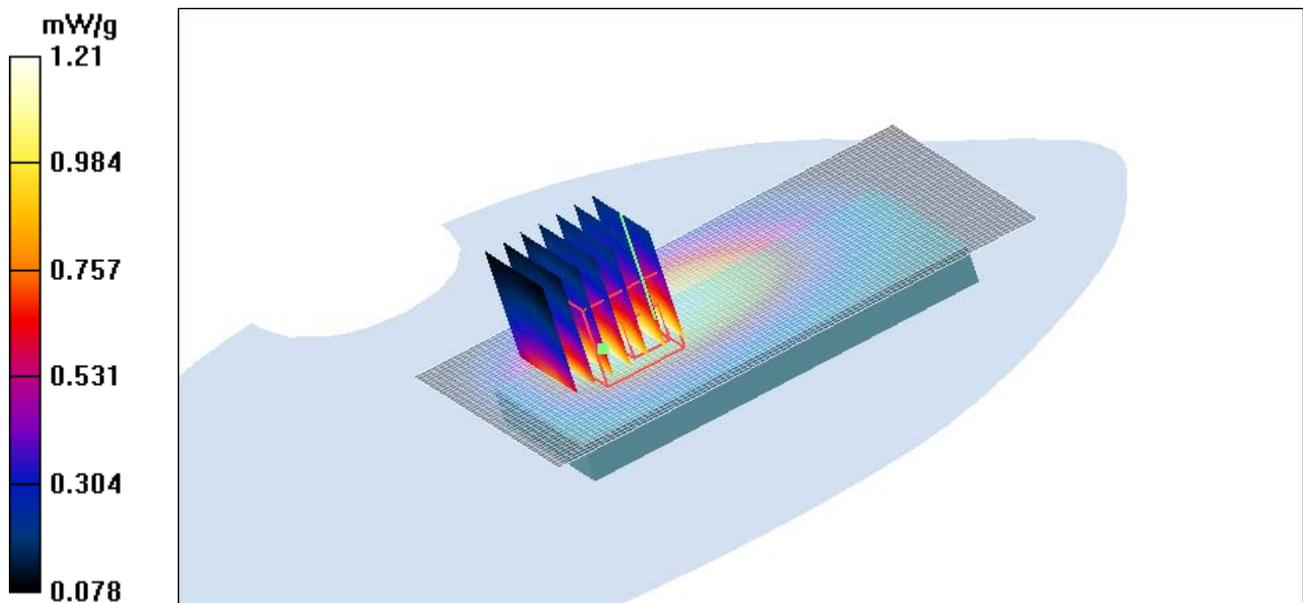
Figure 35 Body, Towards Ground, CDMA Cellular Channel 384
