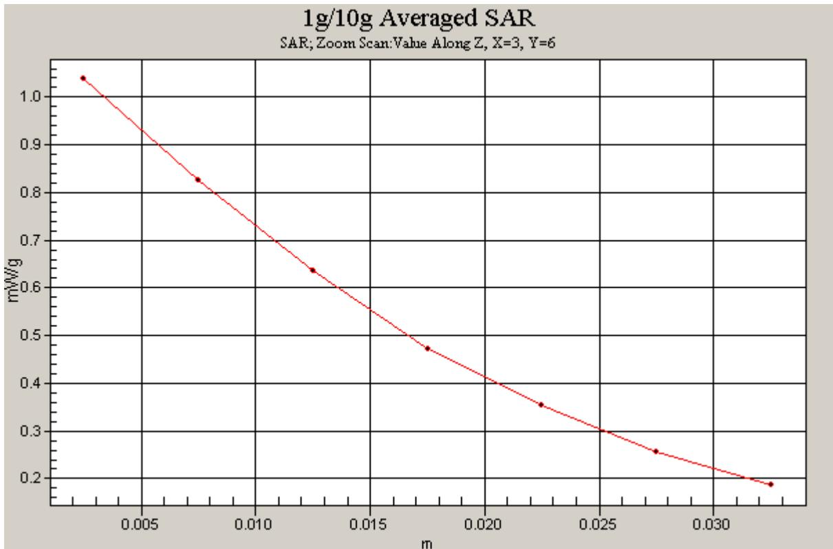
Figure 22 Z-Scan at power reference point (Right Hand Touch Cheek CDMA Cellular Channel 777)
