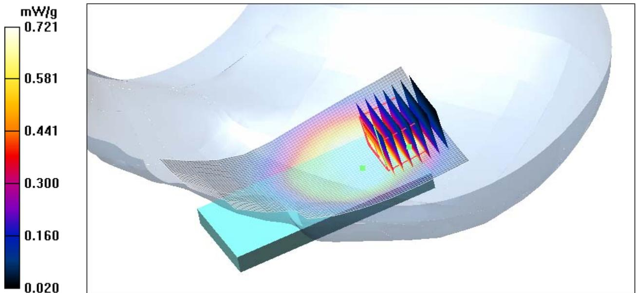
Figure 13 Left Hand Touch Cheek CDMA Cellular Channel 1013
