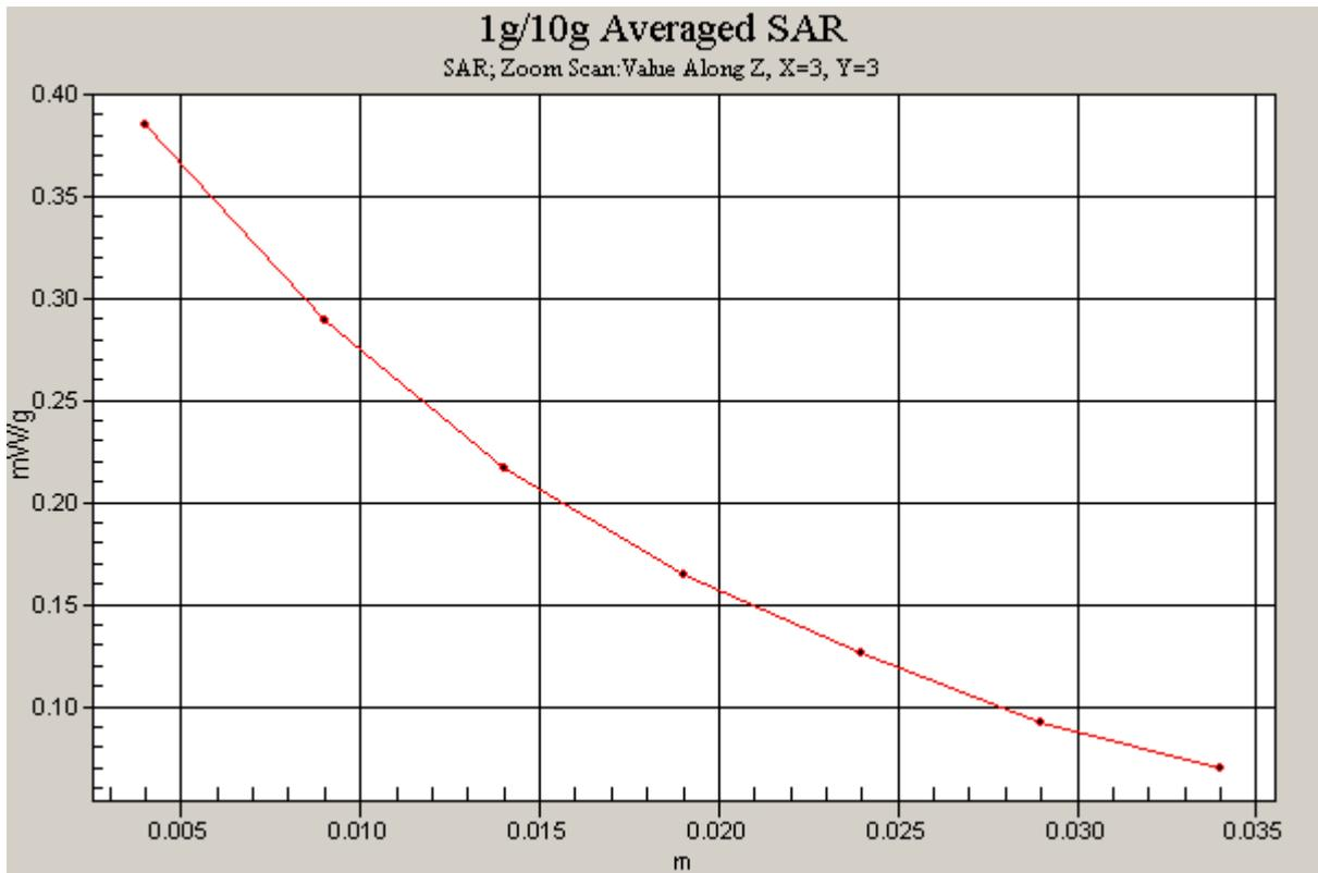
Figure 44 Z-Scan at power reference point (Body, Towards Phantom, , CDMA Cellular Channel 1013)
