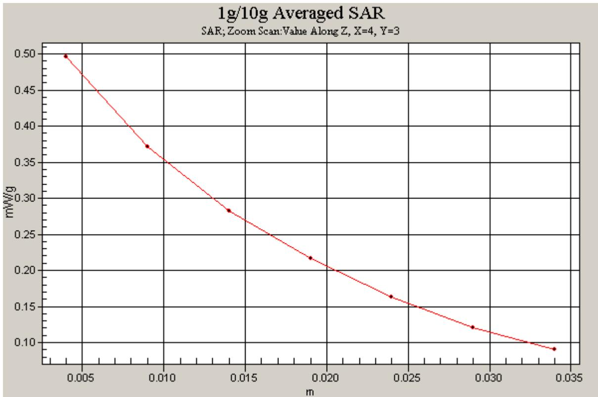
Figure 42 Z-Scan at power reference point (Body, Towards Phantom, , CDMA Cellular Channel 384)
