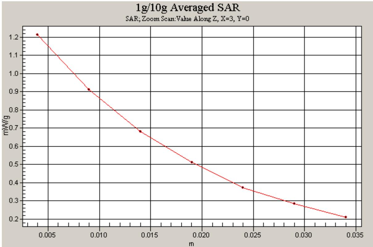
Figure 36 Z-Scan at power reference point (Body, Towards Ground, CDMA Cellular Channel 384)
