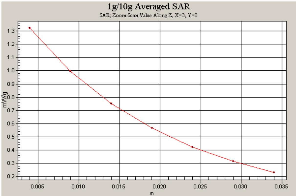
Figure 38 Z-Scan at power reference point (Body, Towards Ground, CDMA Cellular Channel 1013)
