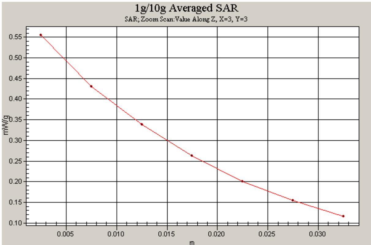
Figure 32 Z-Scan at power reference point (Right Hand Tilt 15°CDMA Cellular Channel 1013)
