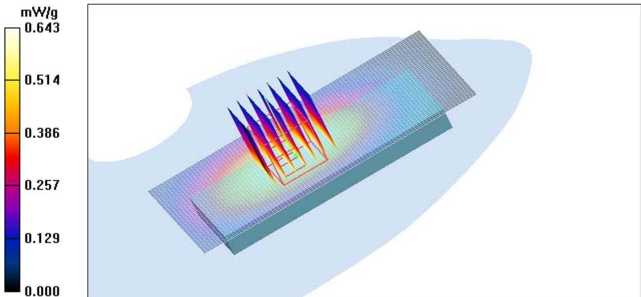
Figure 39 Body, Towards Phantom, CDMA Cellular Channel 777
