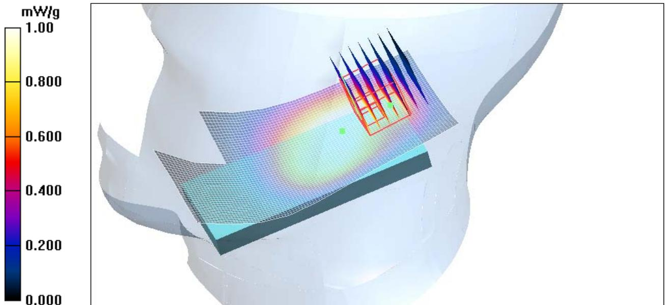
Figure 23 Right Hand Touch Cheek CDMA Cellular Channel 384
