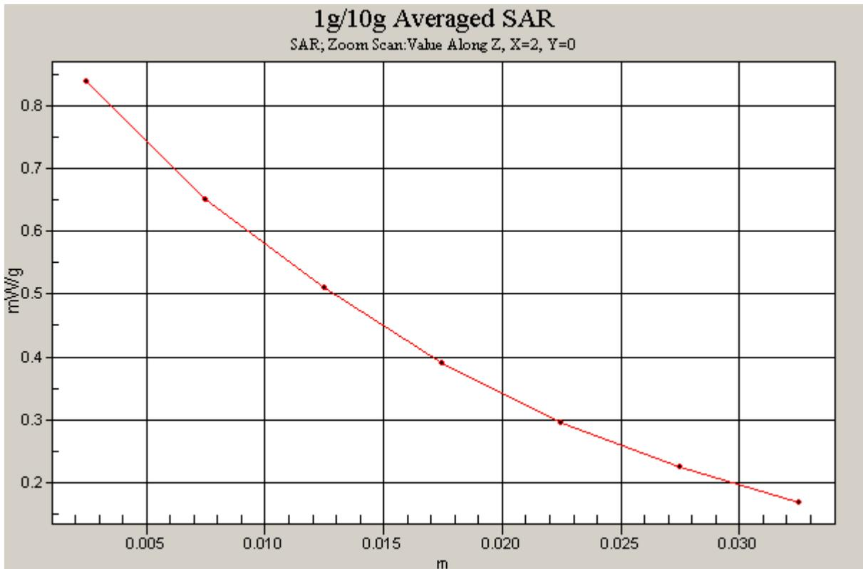
Figure 26 Z-Scan at power reference point (Right Hand Touch Cheek CDMA Cellular Channel 1013)
