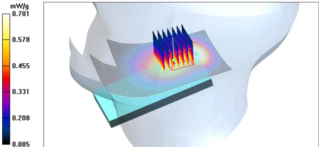
Figure 29 Right Hand Tilt 15°CDMA Cellular Channel 384
