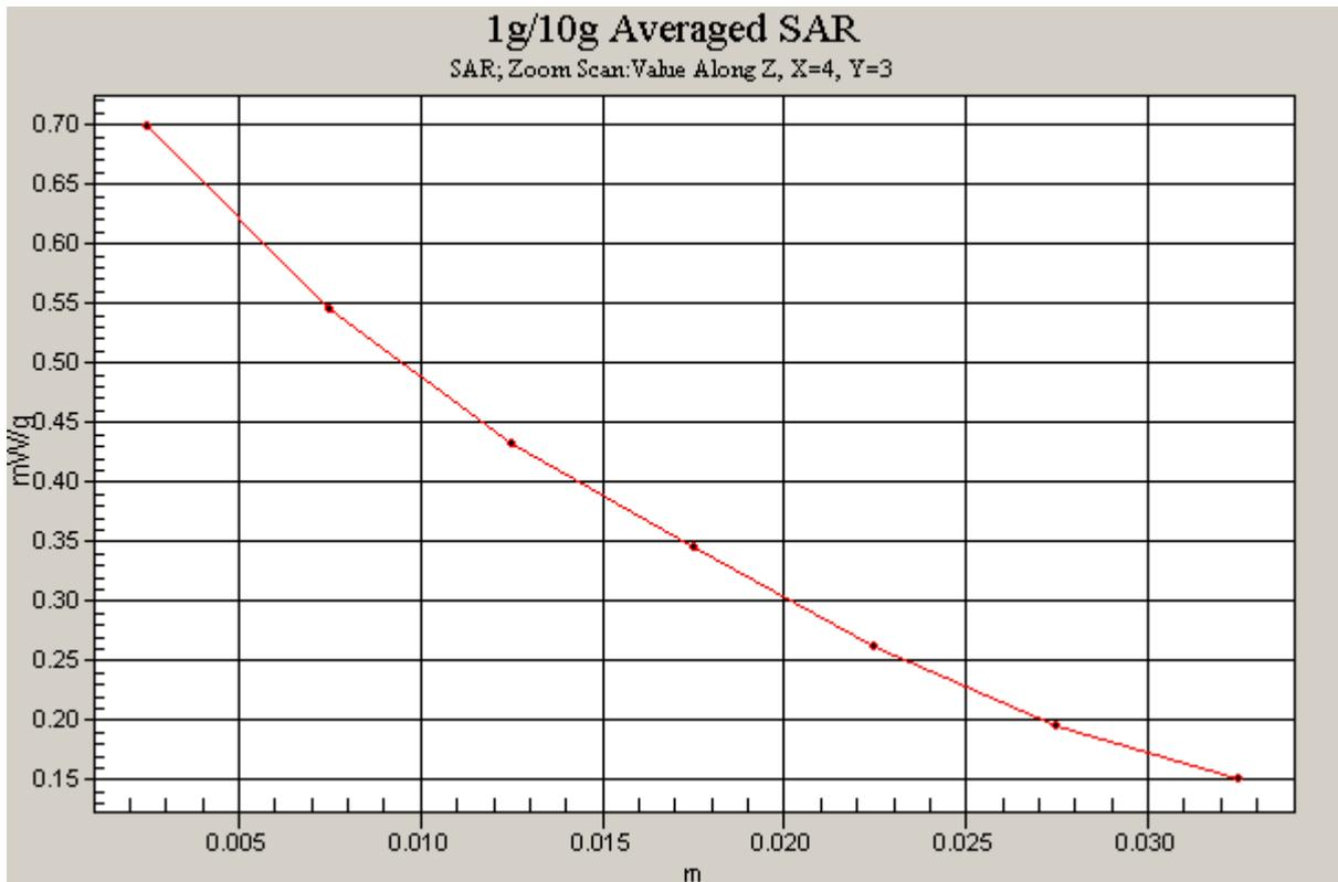
Figure 16 Z-Scan at power reference point (Left Hand Tilt 15°CDMA Cellular Channel 777)
