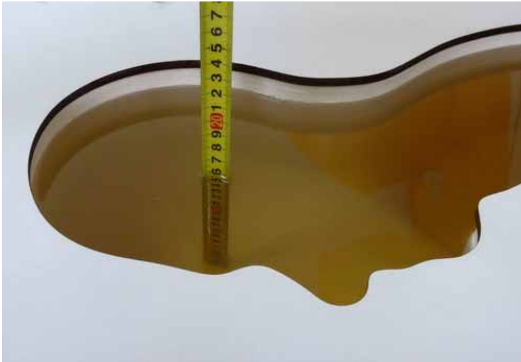
Picture 3: Liquid depth in the head Phantom (835 MHz)
