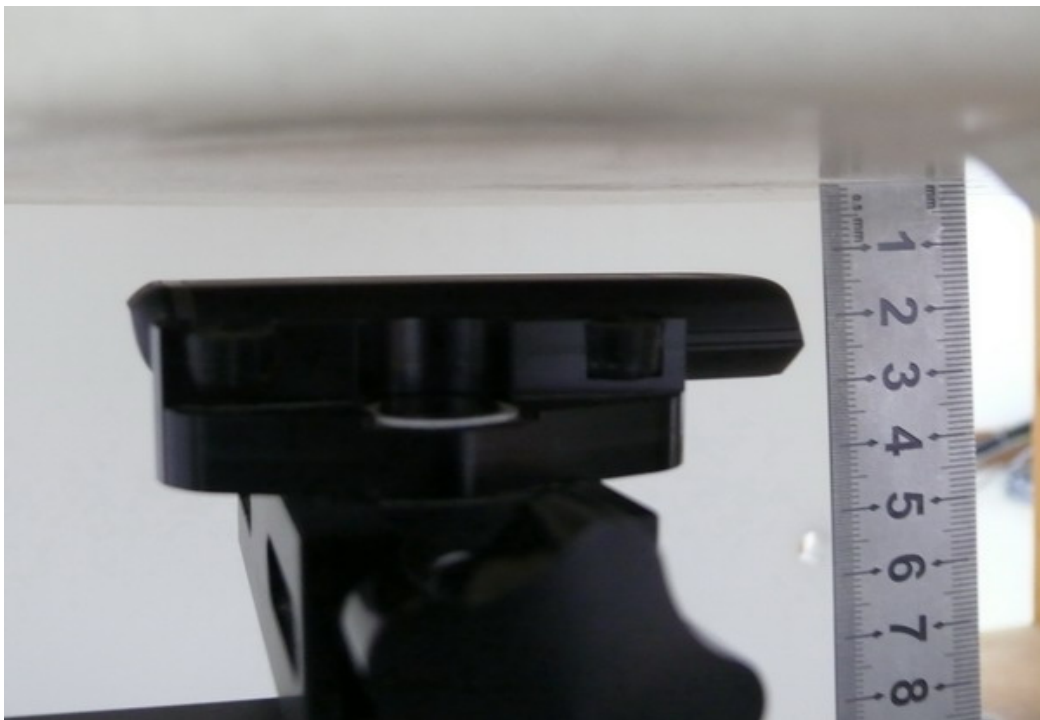
Picture 8: Body, The EUT display towards ground, the distance from handset to the bottom of the Phantom is 15mm)
