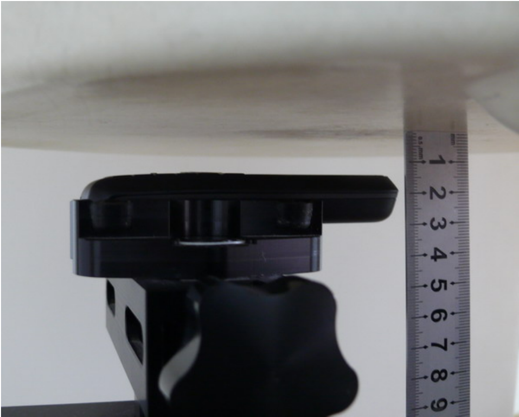
Picture 9: Body, The EUT display towards the Phantom, the distance from handset to the bottom of the Phantom is 15mm)
