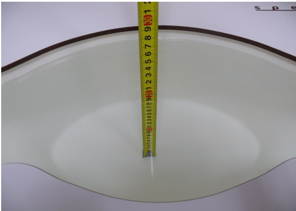
Picture 2: Liquid depth in the Flat Phantom (1900 MHz)
