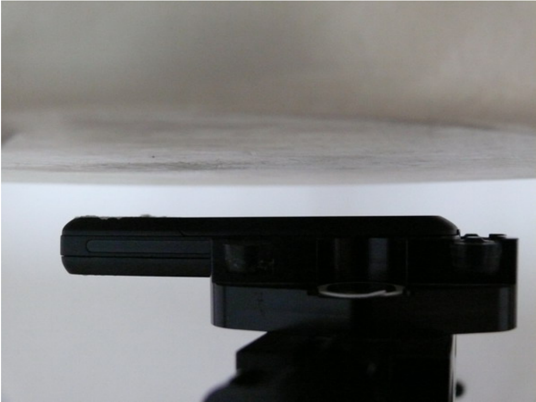
Picture 8: Body, Towards Ground, the distance from handset to the bottom of the Phantom is 15mm)
