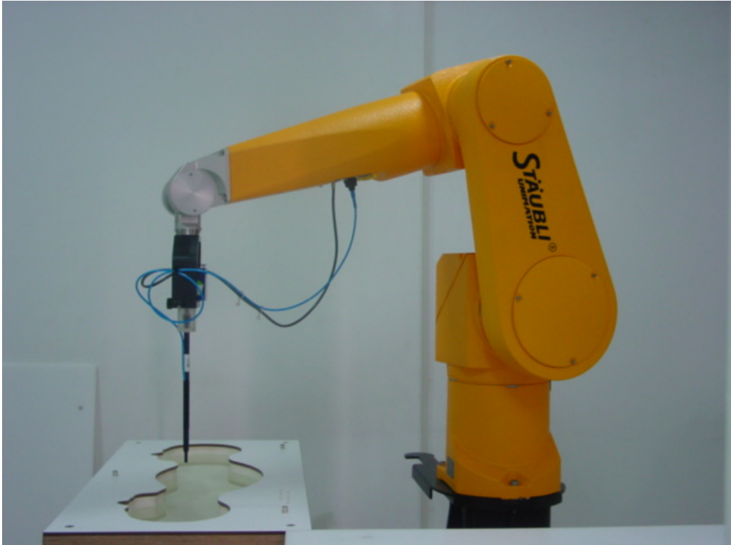
Picture 2: Specific Absorption Rate Test Layout
