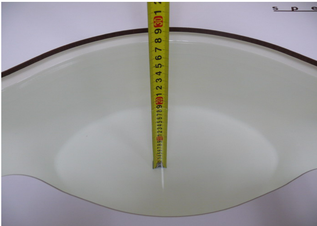
Picture 3: Liquid depth in the Flat Phantom (1900 MHz)
