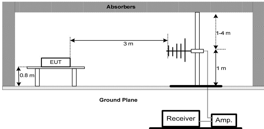
(B) Radiated Emission Test Set-Up Frequency 1 GHz-18GHz
