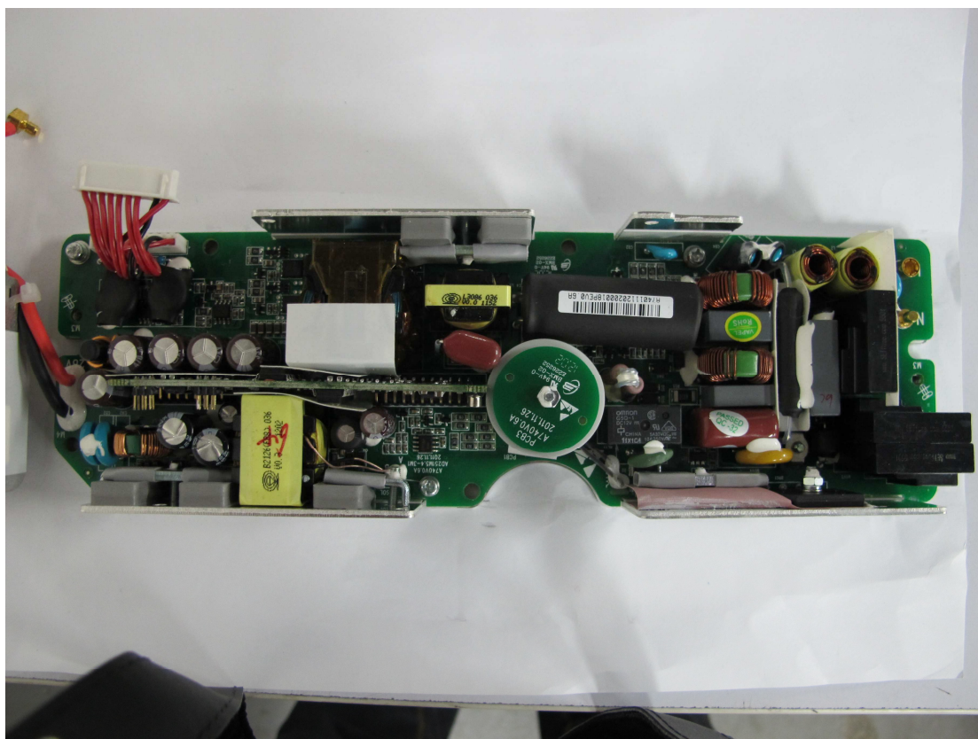
Photo-07 Internal View - Power Board with "VAPEL" Log (internal)
