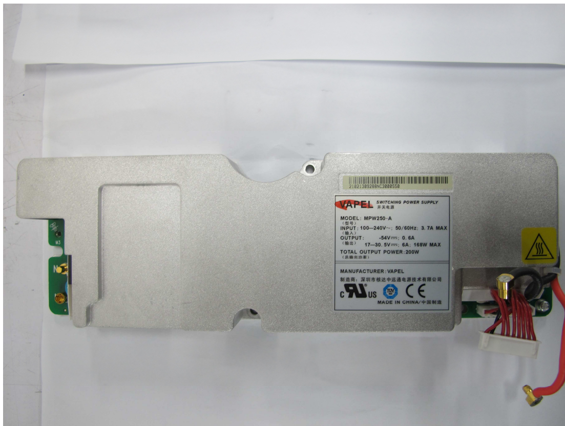
Photo-06 Internal View - Power Board with "VAPEL" Log (external)
