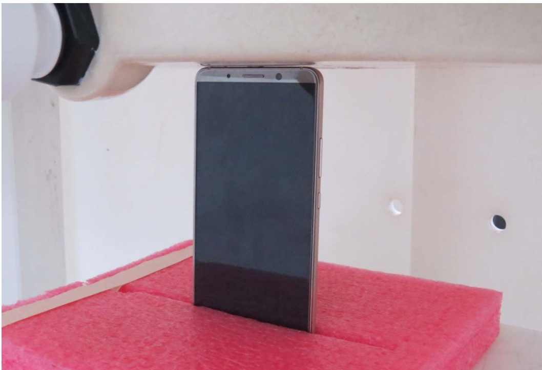
Picture 20: Top Side, the distance from handset to the bottom of the Phantom is 0mm
