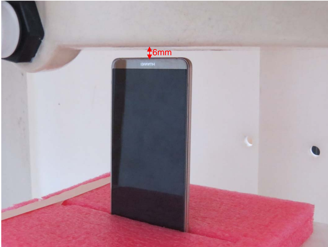
Picture 15: Bottom Side, the distance from handset to the bottom of the Phantom is 6mm
