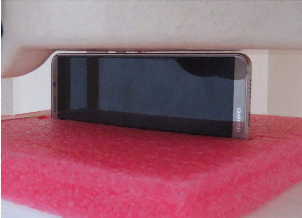
Picture 40: Right Side, the distance from handset to the bottom of the Phantom is 0mm
