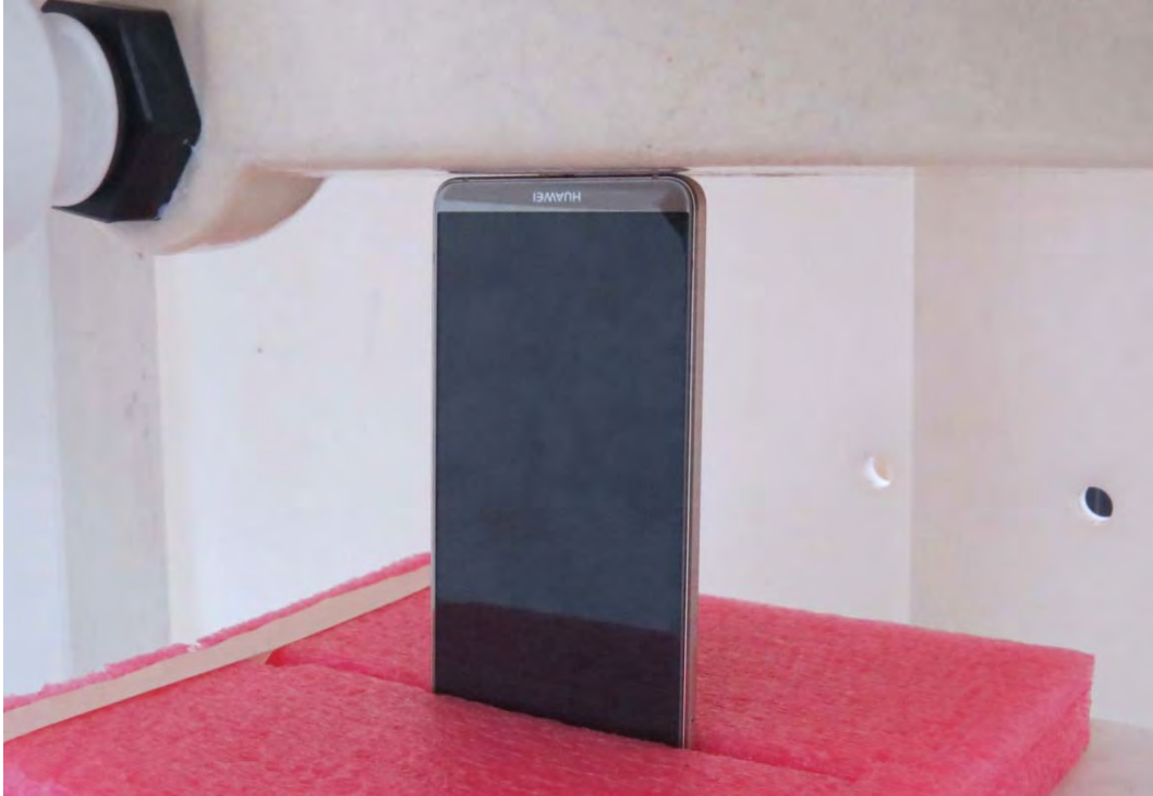
Picture 42: Bottom Side, the distance from handset to the bottom of the Phantom is 0mm
