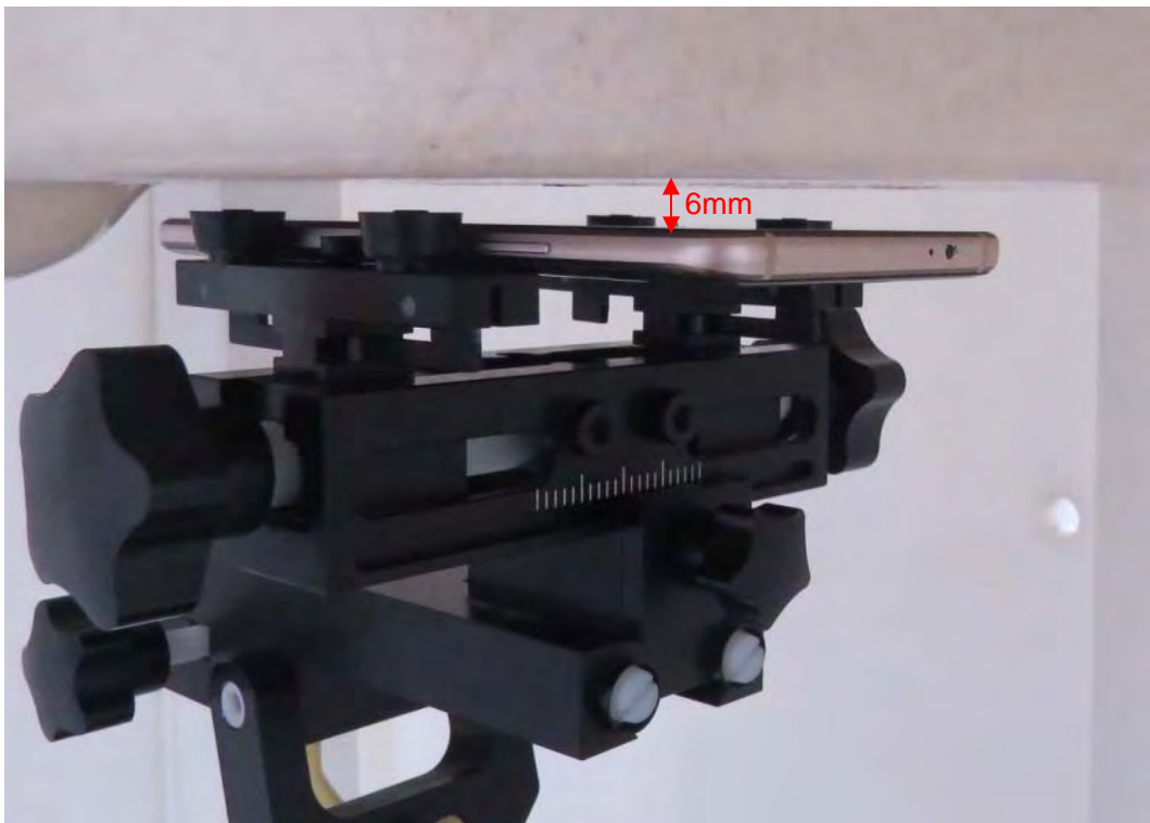
Picture 35: Front Side, the distance from handset to the bottom of the Phantom is 6mm
