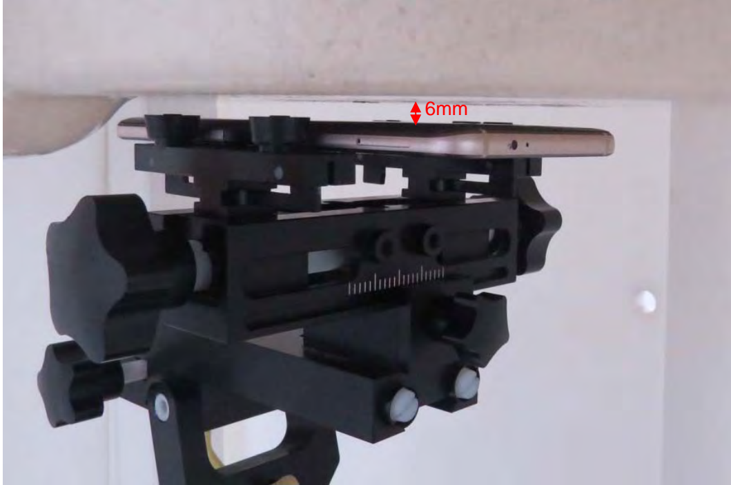
Picture 34: Back Side, the distance from handset to the bottom of the Phantom is 6mm
