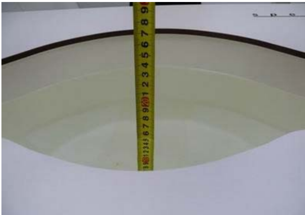
Picture 4: Liquid depth in the flat Phantom
