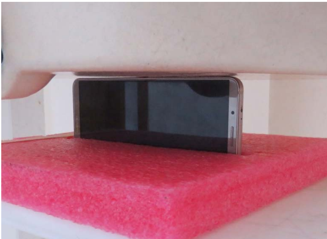
Picture 18: Left Side, the distance from handset to the bottom of the Phantom is 0mm
