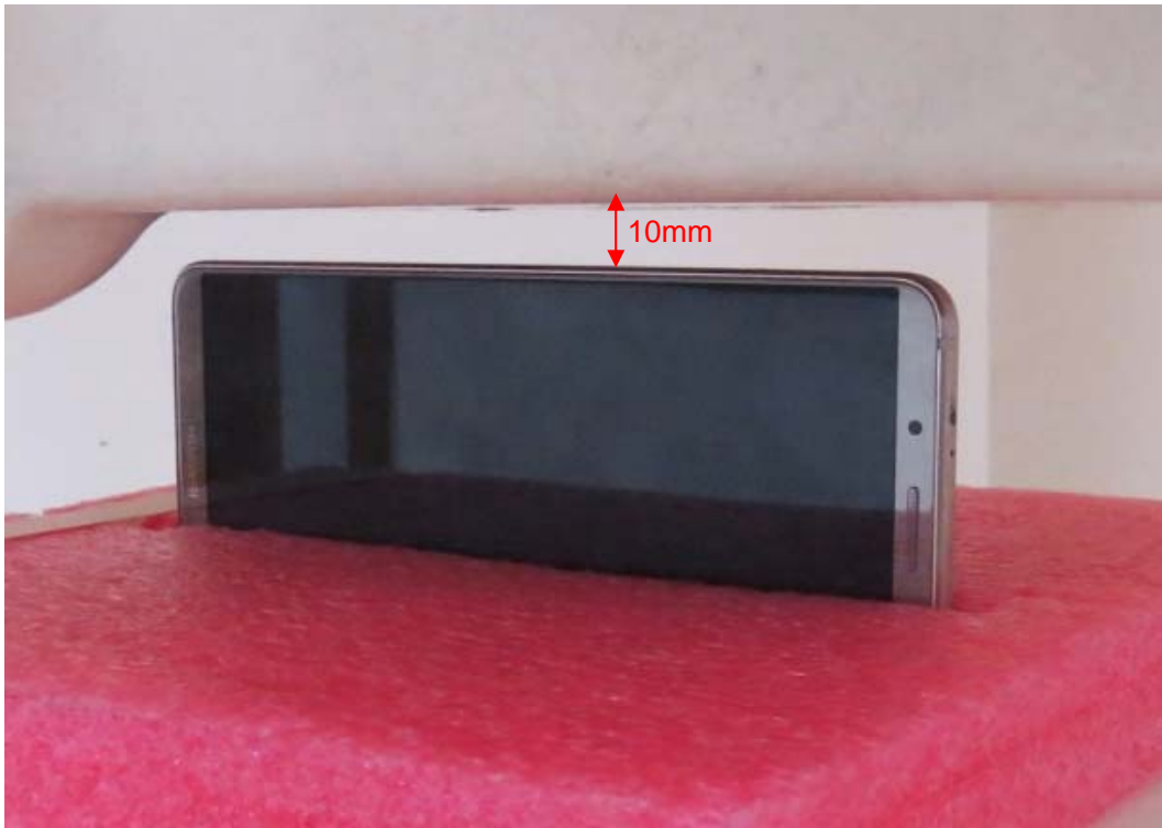
Picture 9: Left Side, the distance from handset to the bottom of the Phantom is 10mm
