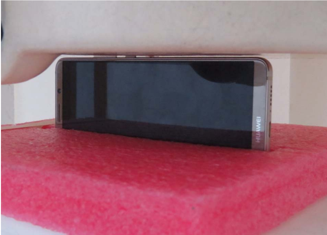
Picture 19: Right Side, the distance from handset to the bottom of the Phantom is 0mm
