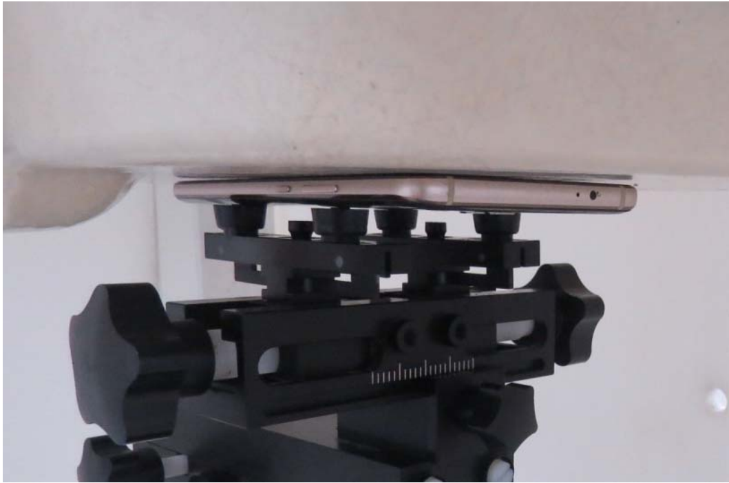
Picture 17: Front Side, the distance from handset to the bottom of the Phantom is 0mm
