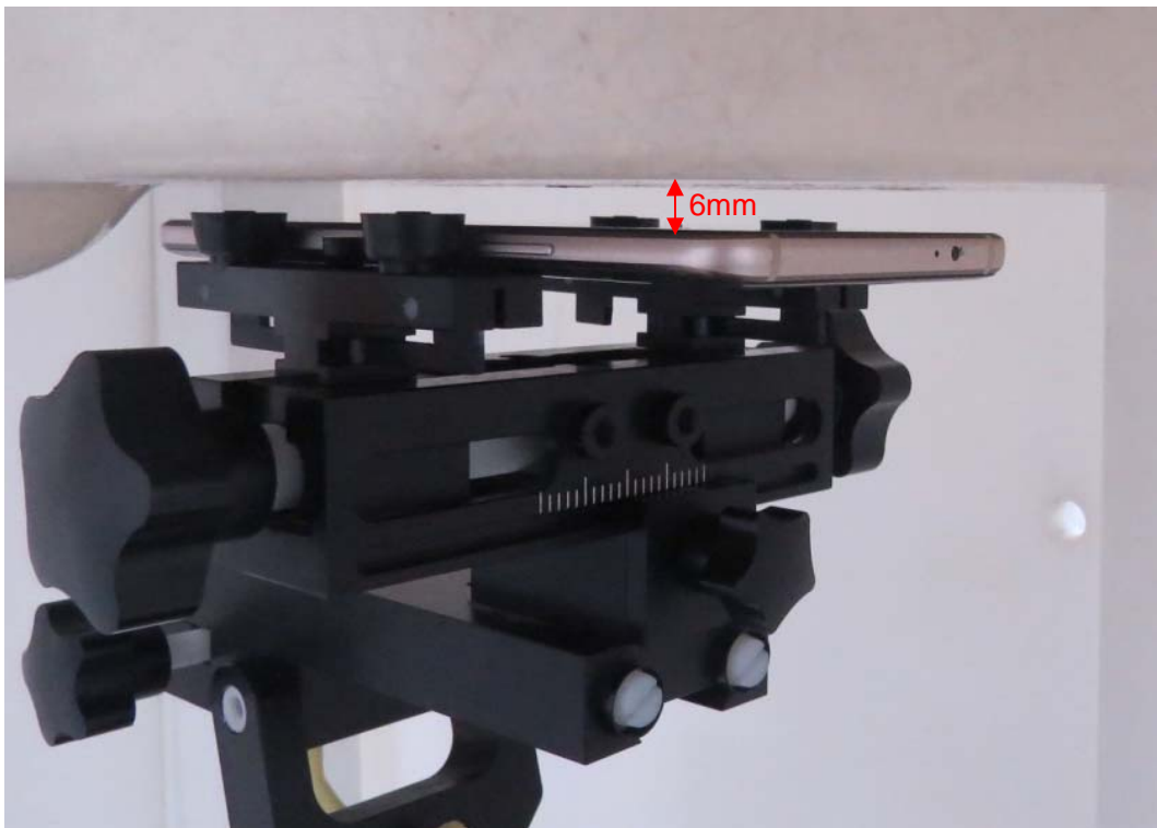
Picture 14: Front Side, the distance from handset to the bottom of the Phantom is 6mm
