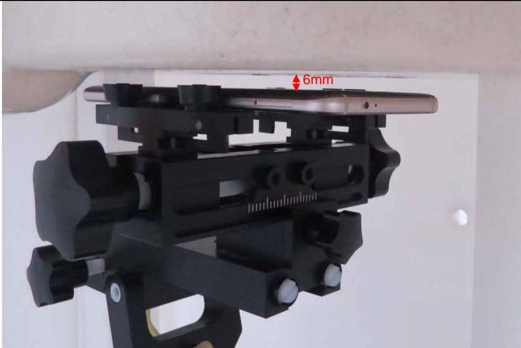
Picture 13: Back Side, the distance from handset to the bottom of the Phantom is 6mm
