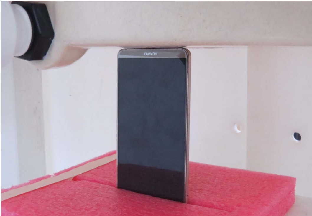
Picture 21: Bottom Side, the distance from handset to the bottom of the Phantom is 0mm
