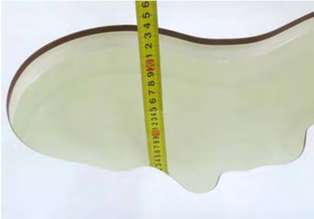
Picture 17: Liquid depth in the head Phantom (5600 MHz, 15.4cm depth)
