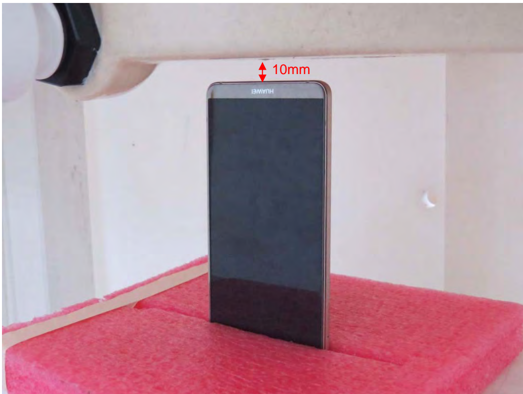
Picture 33: Bottom Side, the distance from handset to the bottom of the Phantom is 10mm
