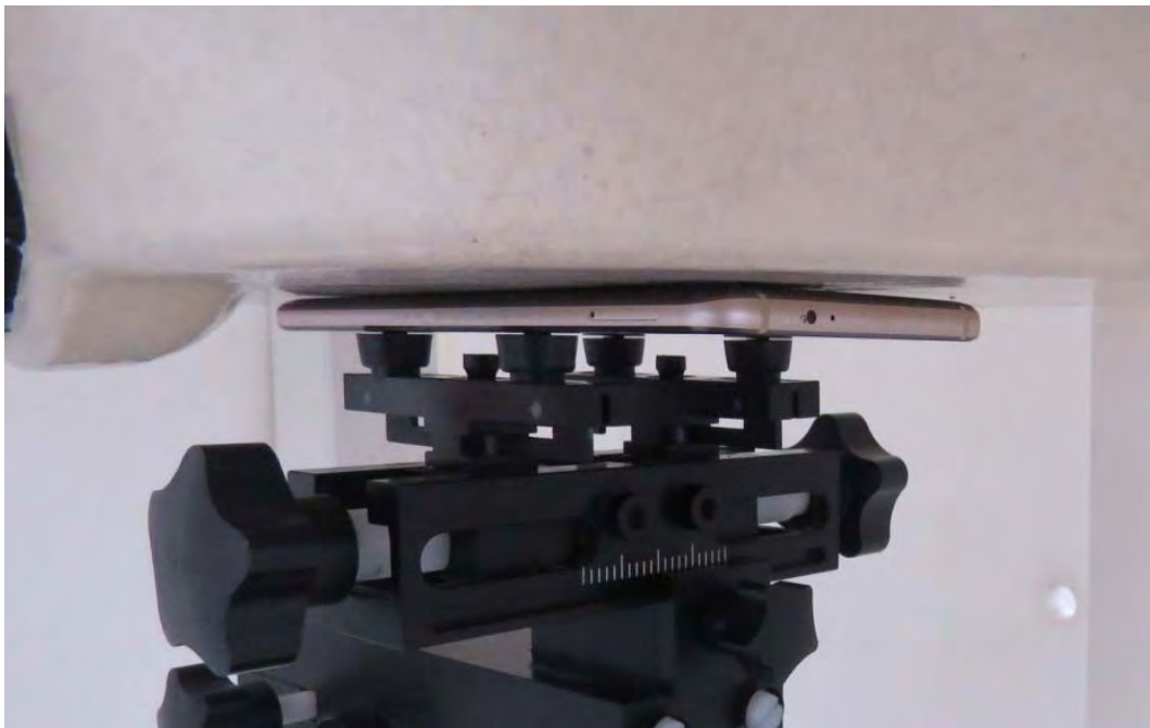
Picture 37: Back Side, the distance from handset to the bottom of the Phantom is 0mm
