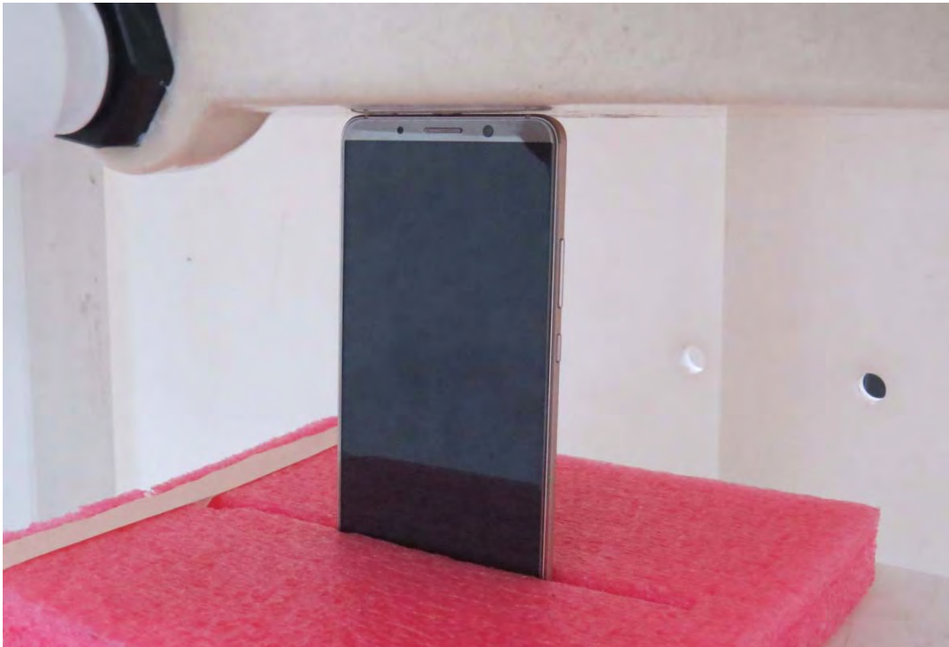
Picture 41: Top Side, the distance from handset to the bottom of the Phantom is 0mm
