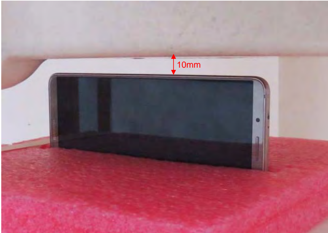
Picture 30: Left Side, the distance from handset to the bottom of the Phantom is 10mm
