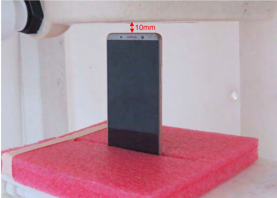
Picture 32: Top Side, the distance from handset to the bottom of the Phantom is 10mm
