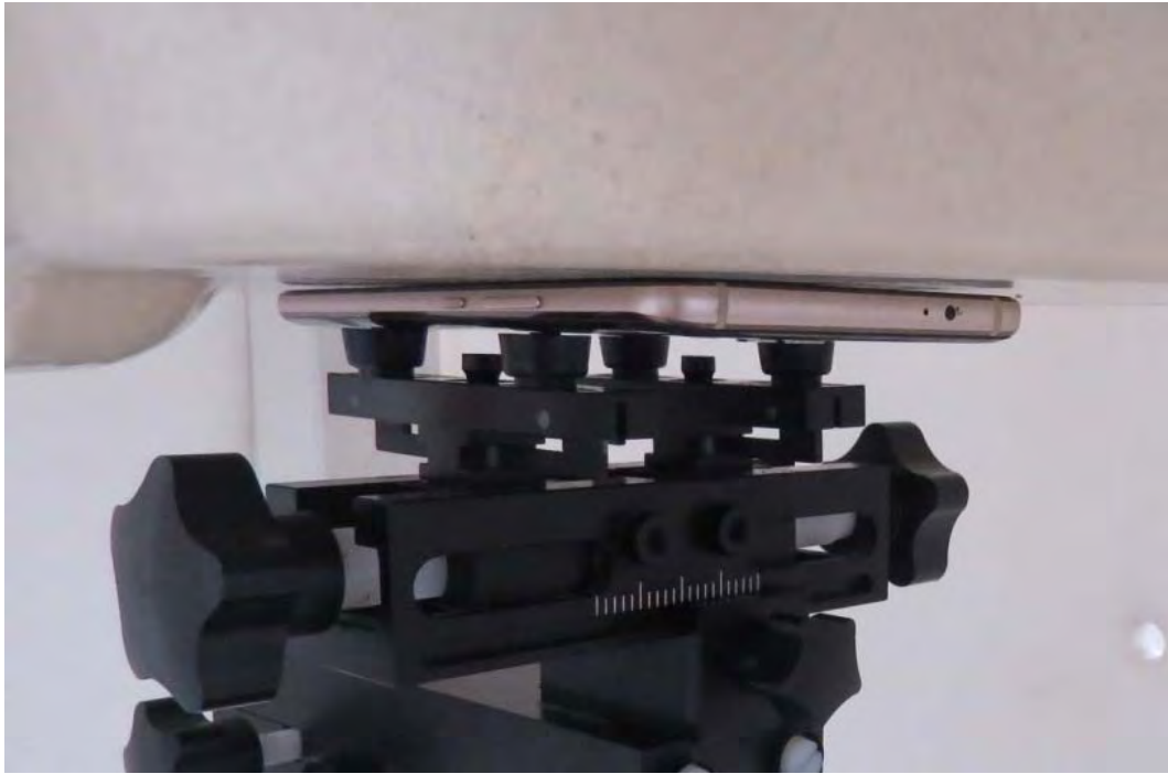
Picture 38: Front Side, the distance from handset to the bottom of the Phantom is 0mm
