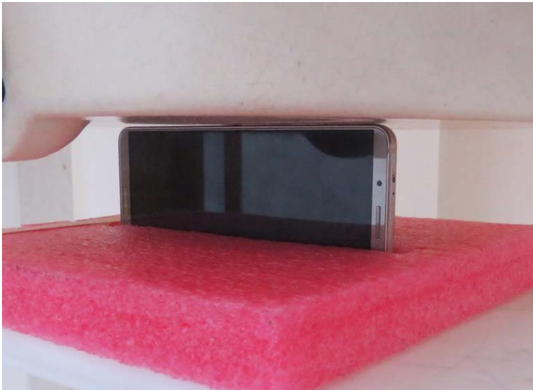
Picture 39: Left Side, the distance from handset to the bottom of the Phantom is 0mm
