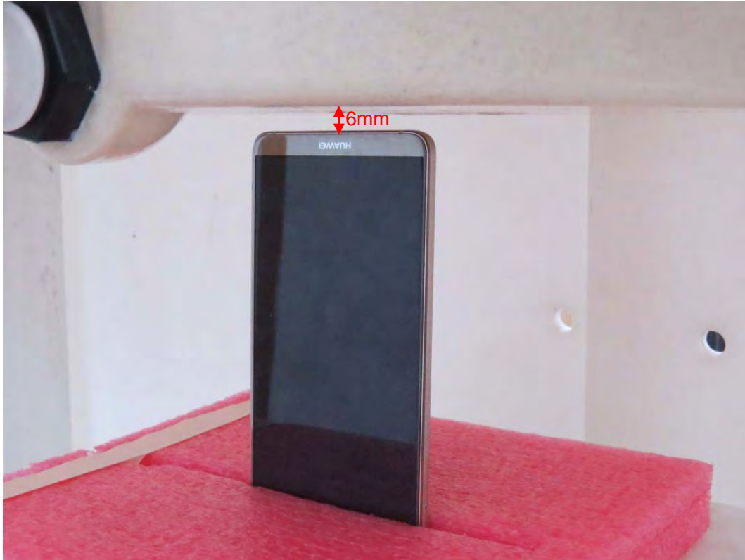
Picture 36: Bottom Side, the distance from handset to the bottom of the Phantom is 6mm
