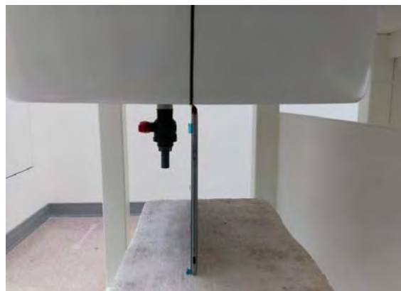
Fig.3 EUT Top side to flat phantom
