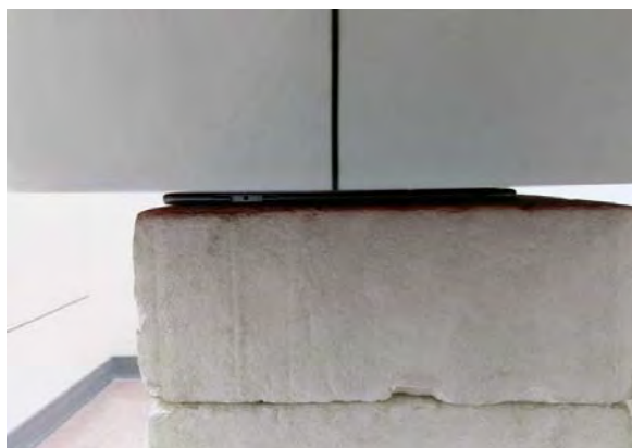
Fig.4 EUT Back side to flat phantom
