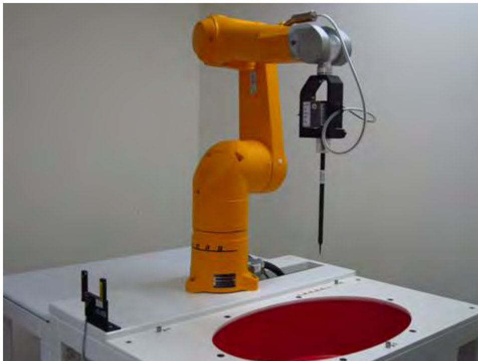
Fig.1 Photograph of the SAR measurement system
