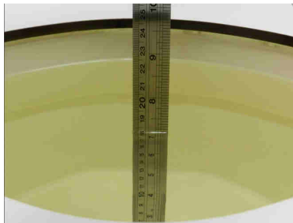
Fig 10.2 Photo of Liquid Height for Body SAR
