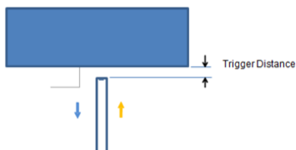
Picture: Proximity sensor triggering distances assessment Bottom Side
