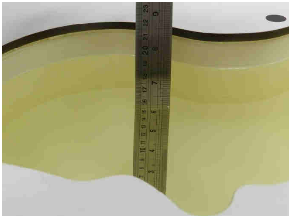
Fig 10.1 Photo of Liquid Height for Head SAR
