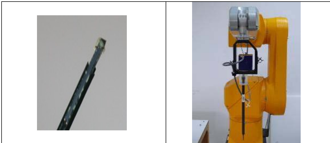
EX3DV4 E-field Probe
