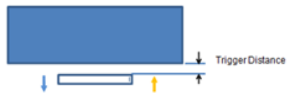
Picture proximity sensor triggering distance assessment Front side and back side
