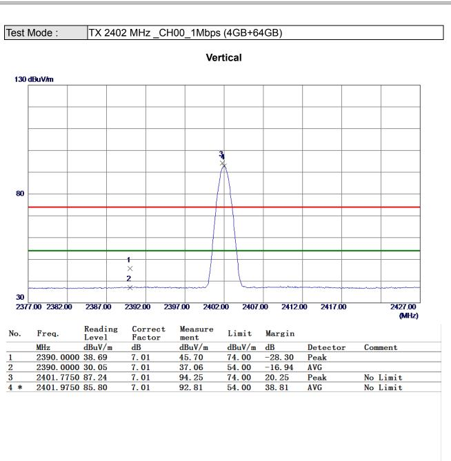
REMARKS: (1) Measurement Value = Reading Level + Correct Factor. (2) Margin Level = Measurement Value - Limit Value.
