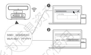
Once the router has connected to a mobile data network, you can connect your computer or mobile phone to the router's Wi-Fi network to access the Internet. Please refer to the label on the back of the router for the default wireless network name (**SSID**) and password (**Wi-Fi KEY**).
