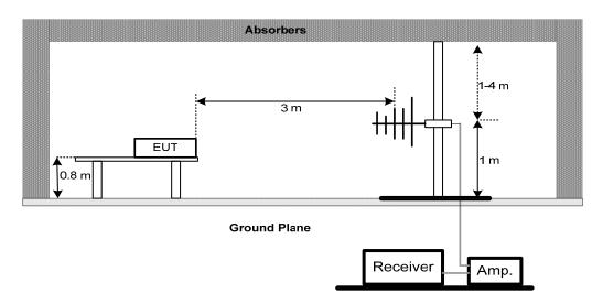
(B) Radiated Emission Test Set-Up Frequency 1-18 GHz
