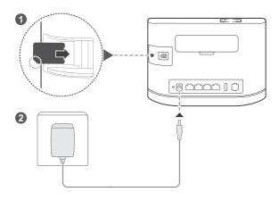
Insert a SIM card into the SIM card slot as shown in the preceding diagram and then connect the power adapter to the B315 router. The router will turn on automatically and search for available mobile networks.
