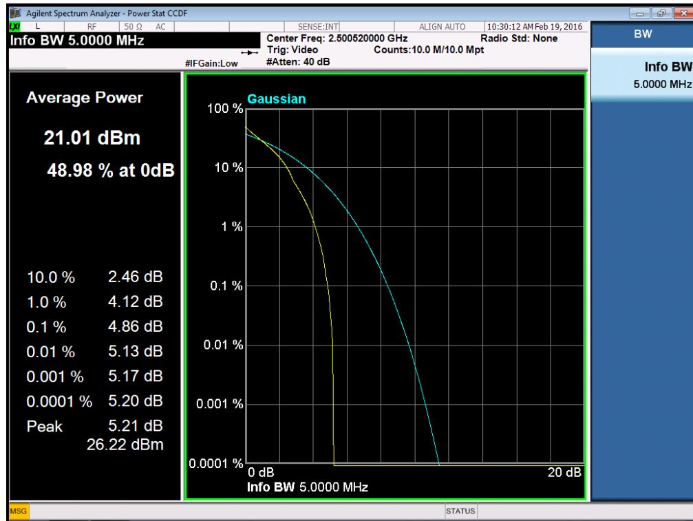
**Peak to Average Ratio of Configuration-LTE Band VII QPSK-5M/1RB
