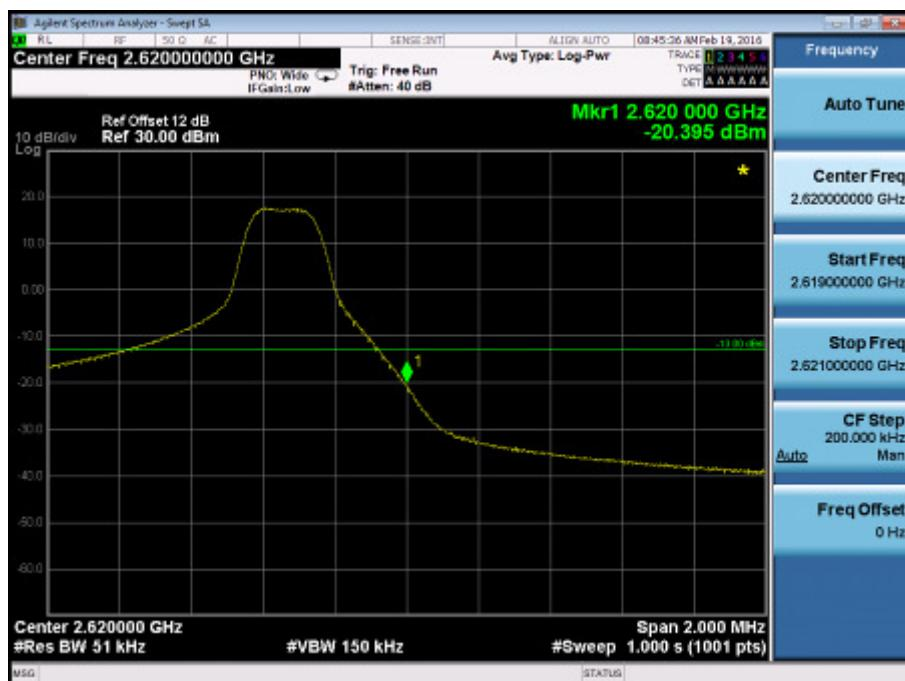
**Band Edge on Configuration LTE Band XXXVIII QPSK-5M / 25RB
