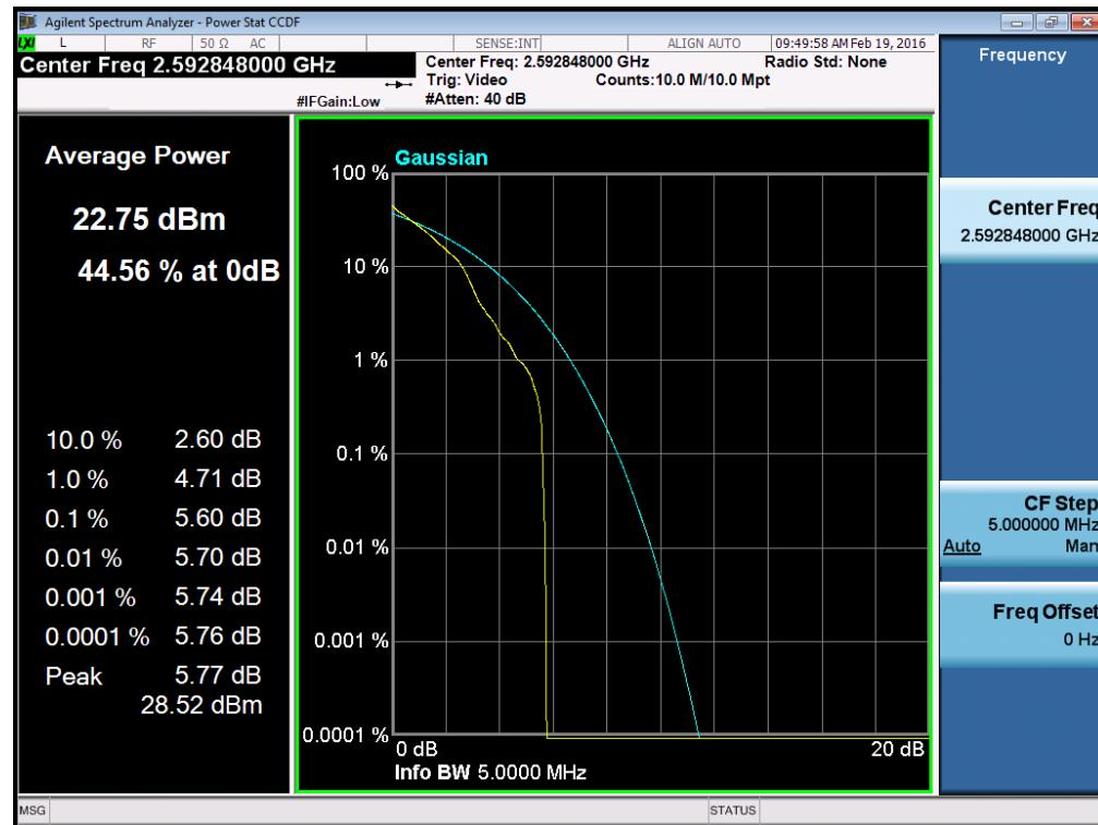
**Peak to Average Ratio of Configuration-LTE Band XXXVIII QPSK-5M/1RB
