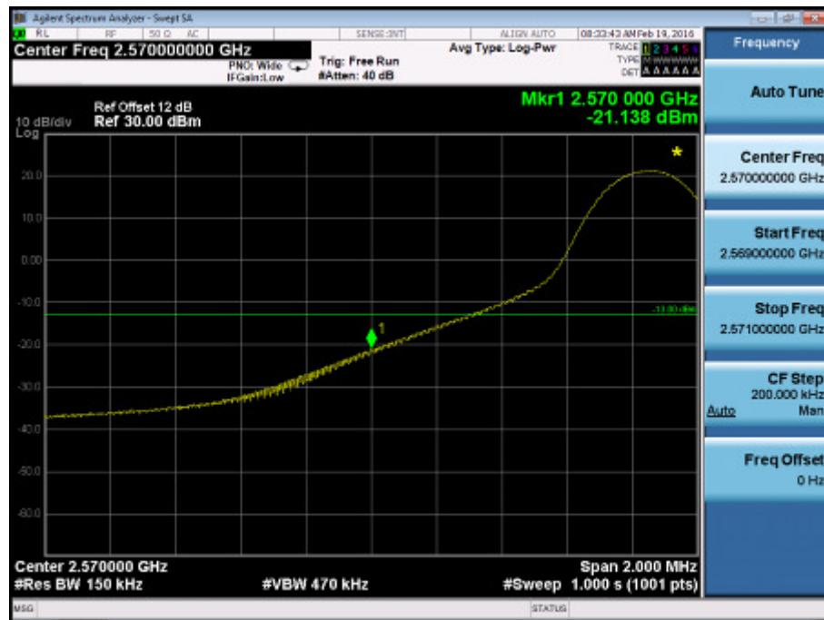
**Band Edge on Configuration LTE Band XXXVIII QPSK-15M / 1RB
