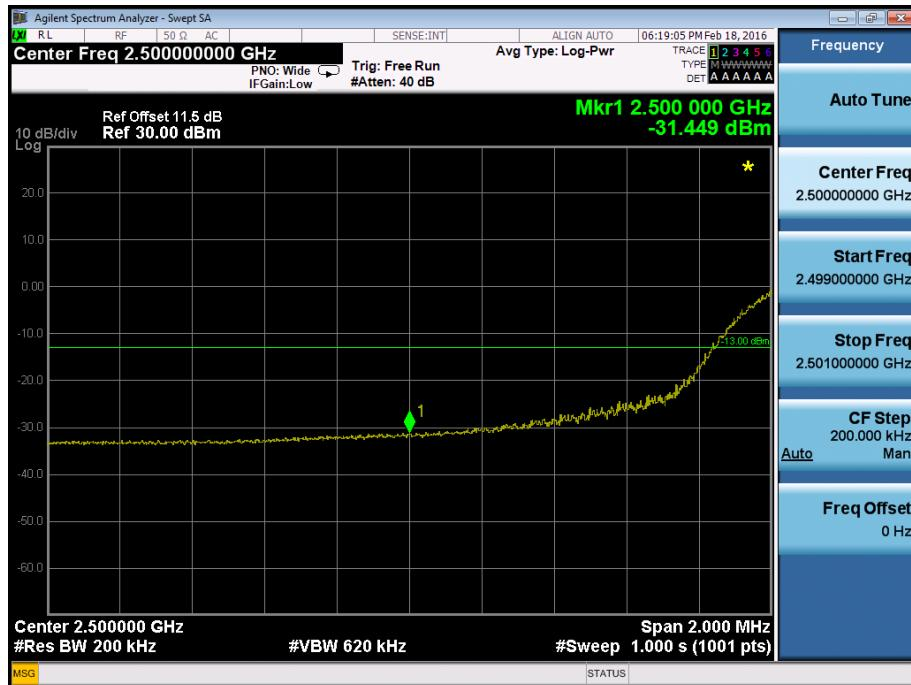
**Band Edge on Configuration LTE Band VII QPSK-20M / 100RB
