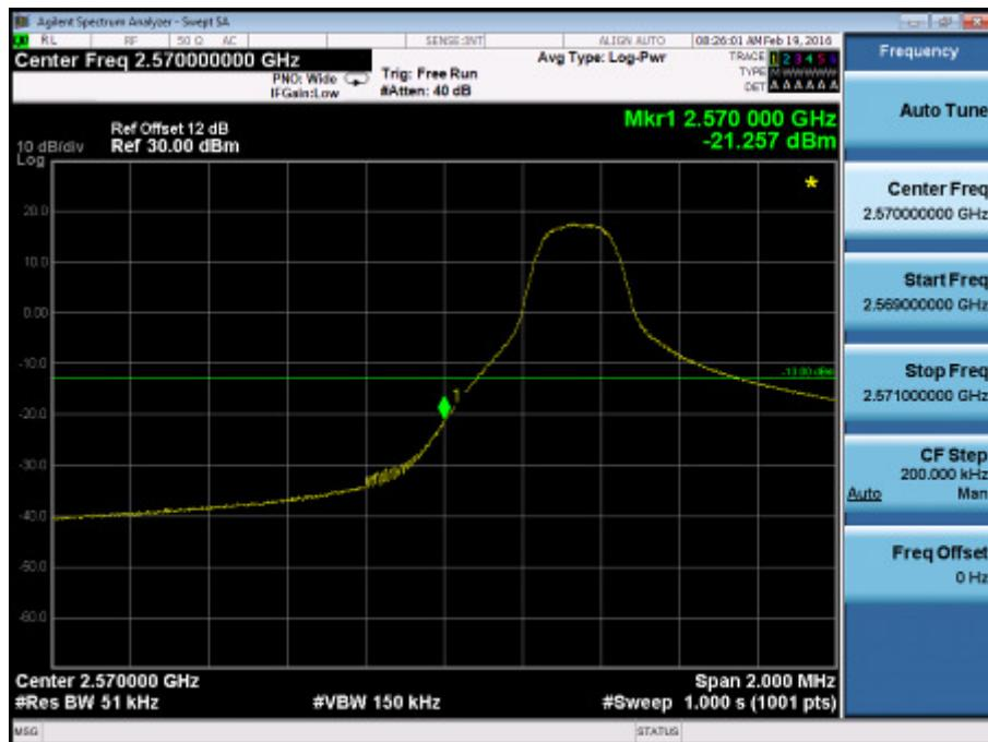
**Band Edge on Configuration LTE Band XXXVIII QPSK-5M / 1RB
