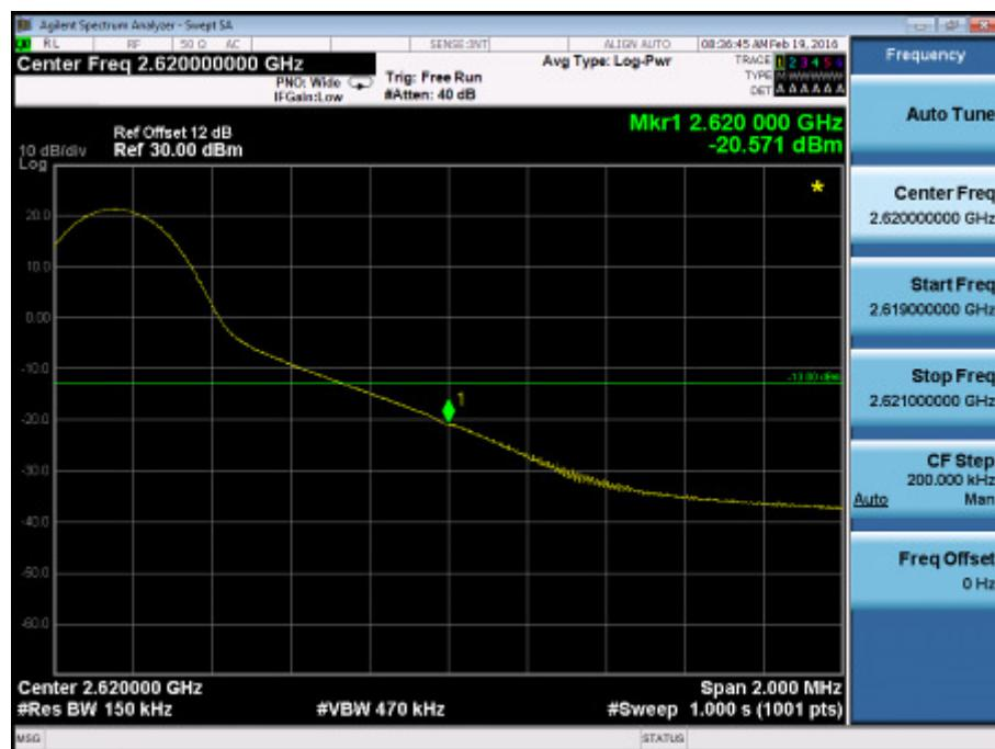
**Band Edge on Configuration LTE Band XXXVIII QPSK-15M / 75RB
