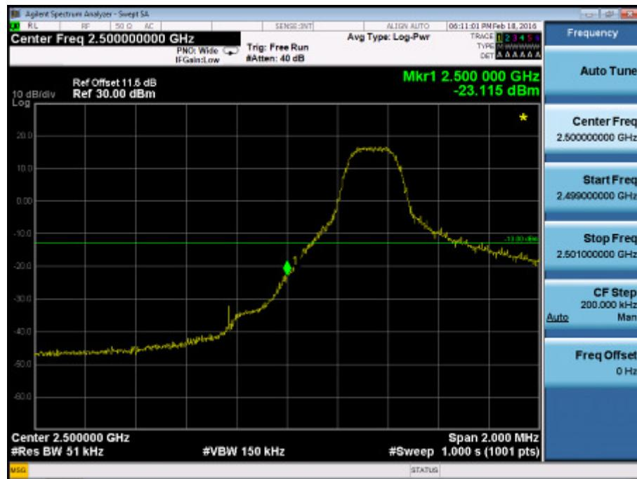
**Band Edge on Configuration LTE Band VII QPSK-5M / 1RB
