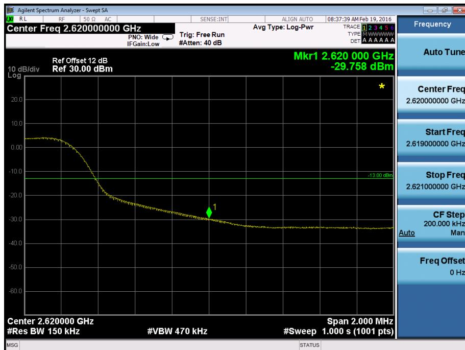
**Band Edge on Configuration LTE Band XXXVIII QPSK-20M / 1RB
