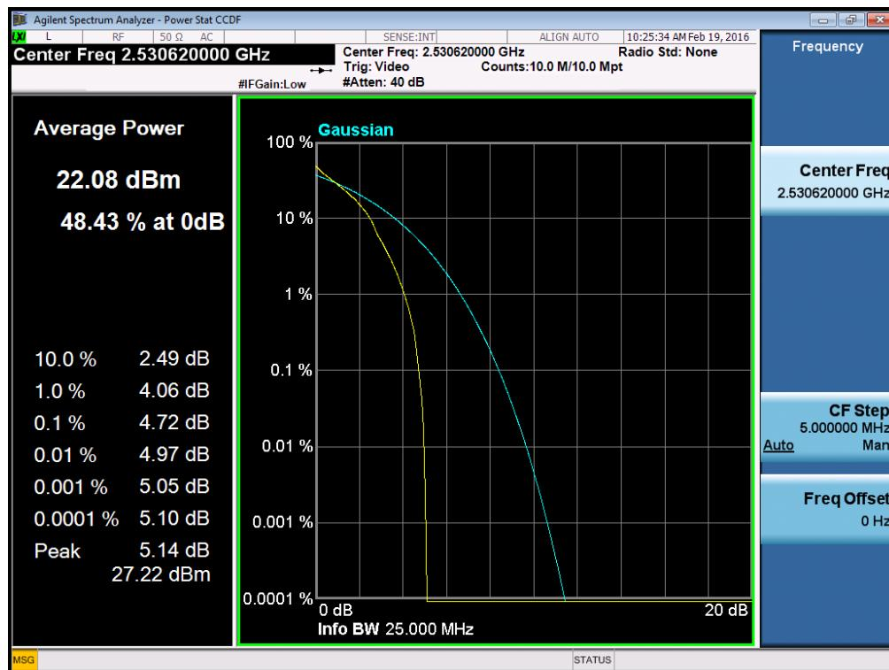
**Peak to Average Ratio of Configuration-LTE Band VII QPSK-10M/1RB
