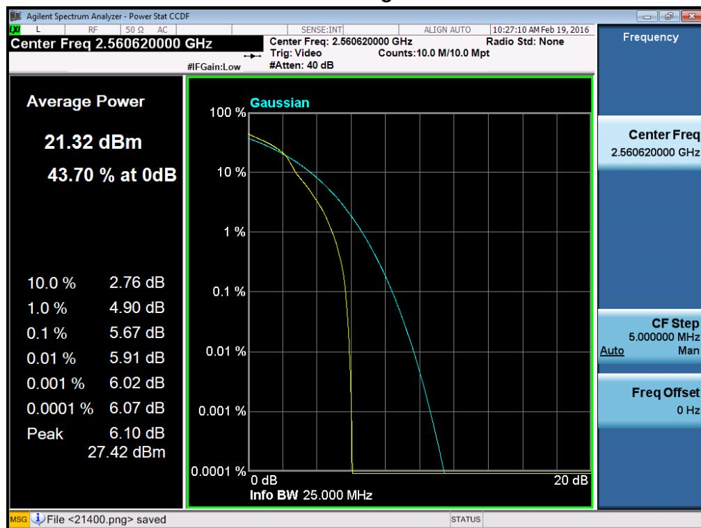
**Peak to Average Ratio of Configuration-LTE Band VII 16-QAM-15M/1RB**
