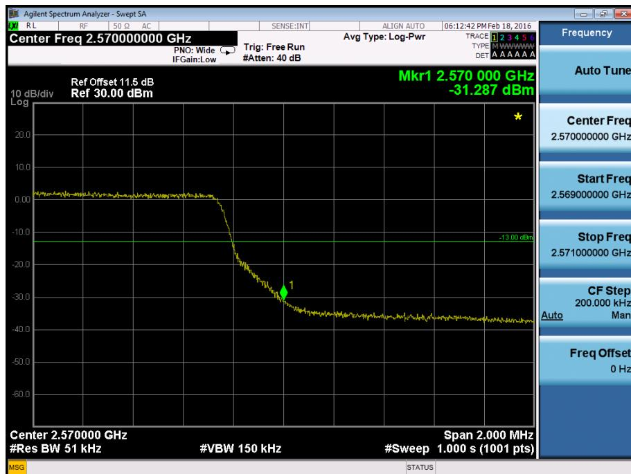
**Band Edge on Configuration LTE Band VII QPSK-10M / 1RB**
