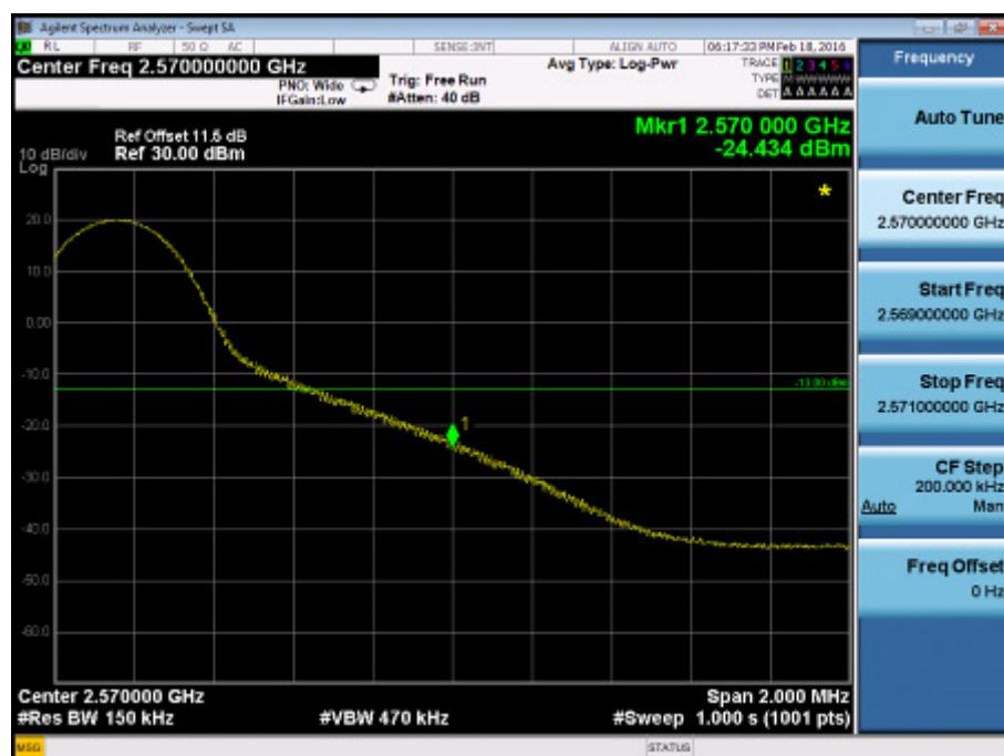
**Band Edge on Configuration LTE Band VII QPSK-15M / 75RB**
