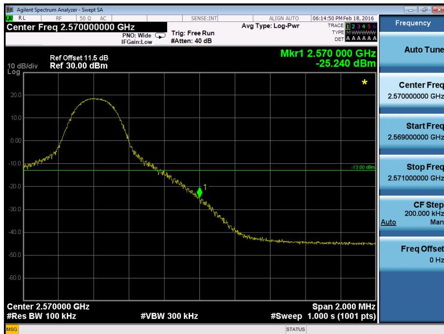
**Band Edge on Configuration LTE Band VII QPSK-10M / 50RB
