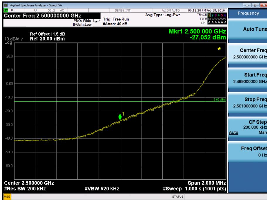
**Band Edge on Configuration LTE Band VII QPSK-20M / 1RB**
