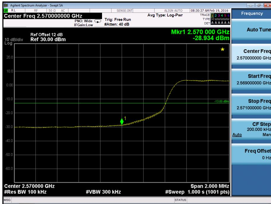
**Band Edge on Configuration LTE Band XXXVIII QPSK-10M / 50RB**
