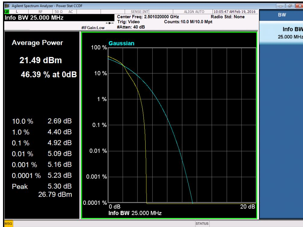
**Peak to Average Ratio of Configuration-LTE Band VII 16-QAM-20M/1RB
