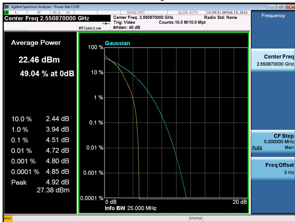
**Peak to Average Ratio of Configuration-LTE Band VII 16-QAM-5M/1RB
