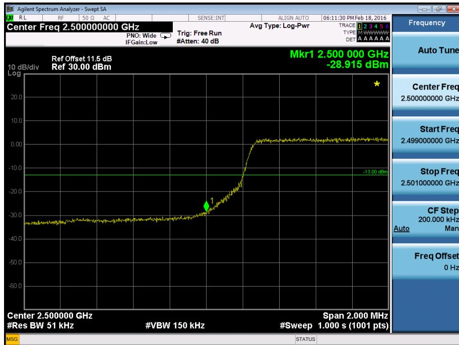
**Band Edge on Configuration LTE Band VII QPSK-5M / 25RB**
