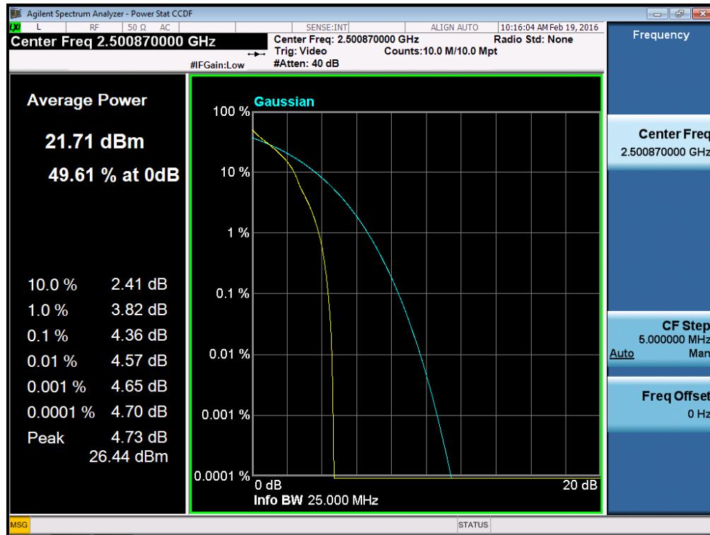
**Peak to Average Ratio of Configuration-LTE Band VII QPSK-15M/1RB
