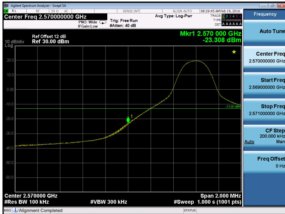
**Band Edge on Configuration LTE Band XXXVIII QPSK-10M / 1RB
