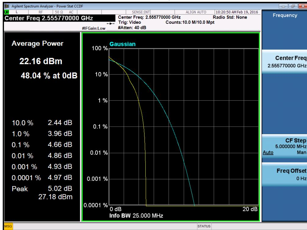
**Peak to Average Ratio of Configuration-LTE Band VII QPSK-20M/1RB
