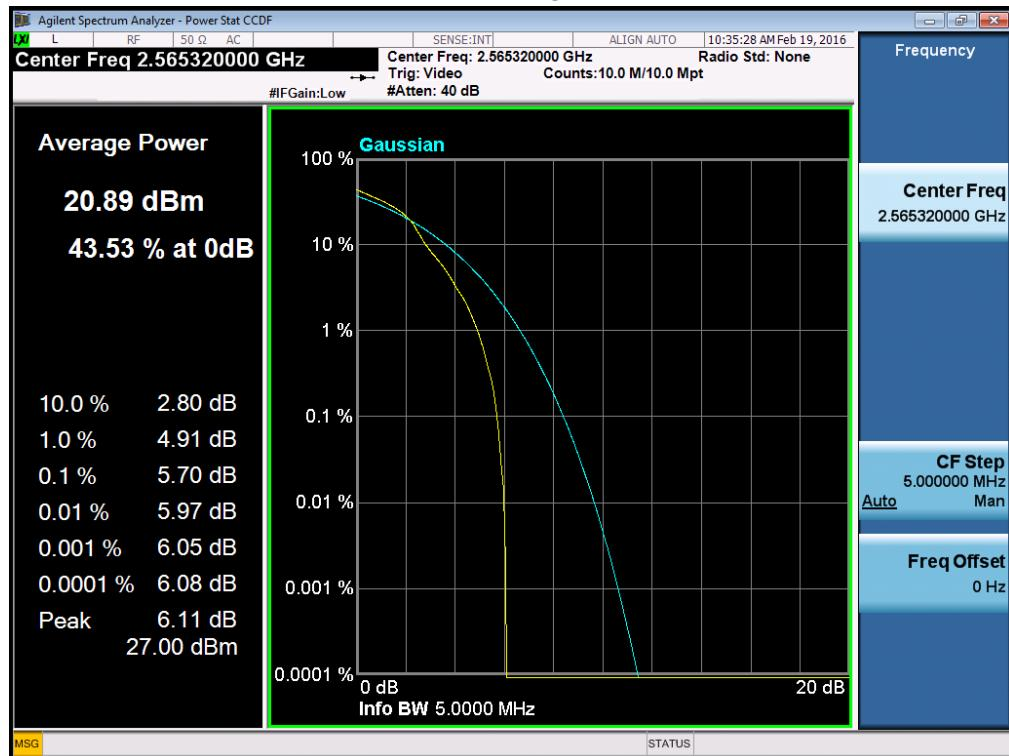
**Peak to Average Ratio of Configuration-LTE Band VII 16-QAM-10M/1RB
