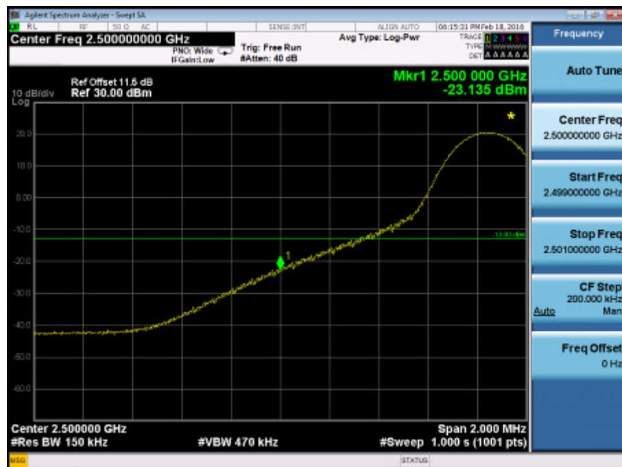
**Band Edge on Configuration LTE Band VII QPSK-15M / 1RB
