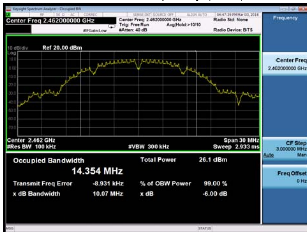
802.11b, Carrier frequency (MHz): 2462
