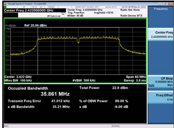
802.11n(HT40), Carrier frequency (MHz): 2437
