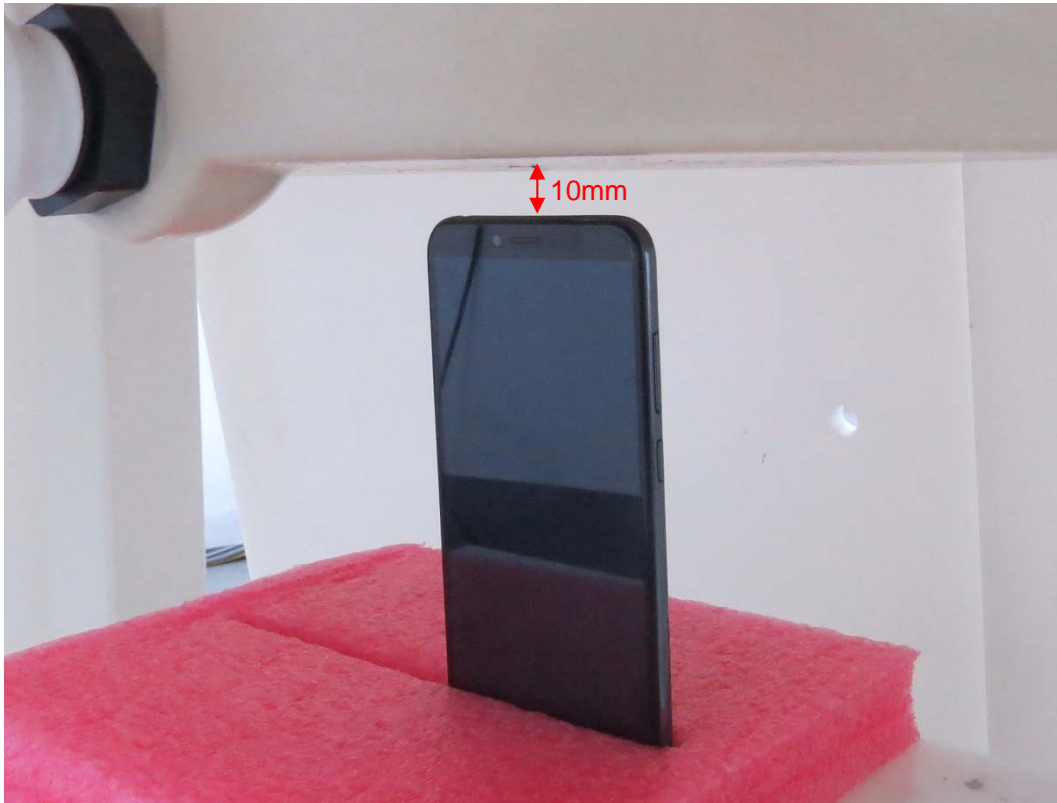
Picture 17: Bottom Side, the distance from handset to the bottom of the Phantom is 10mm (ATU-L21)
