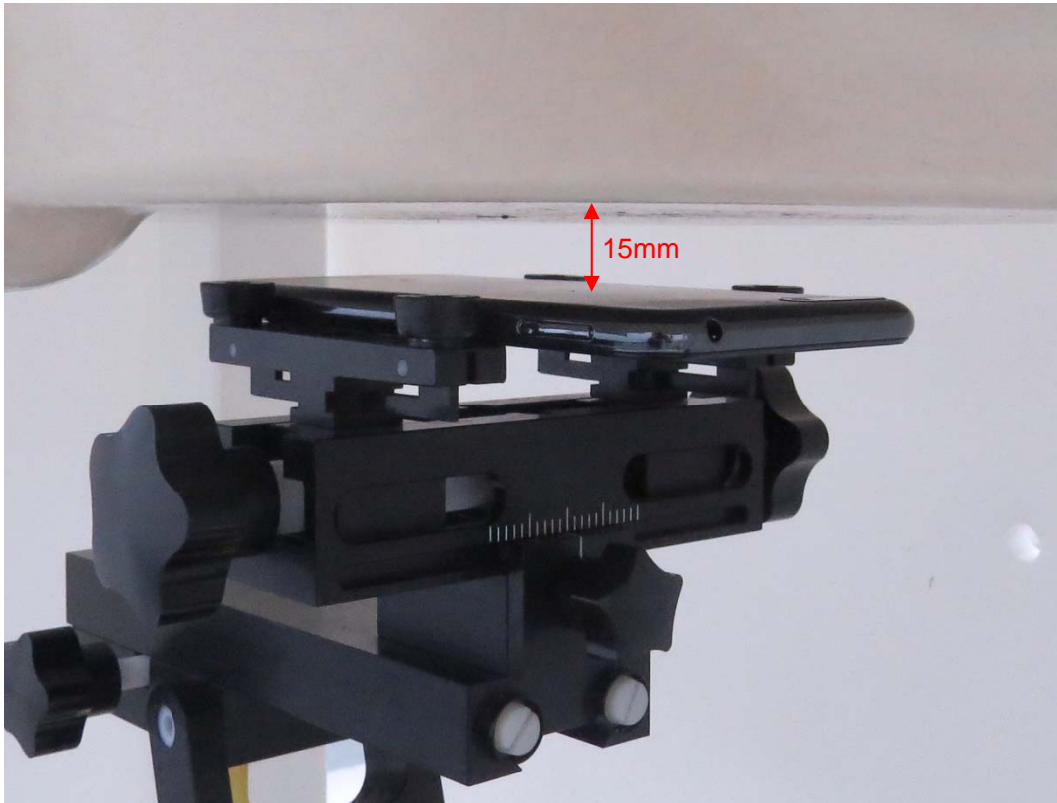
Picture 15: Back Side, the distance from handset to the bottom of the Phantom is 15mm (ATU-L21)
