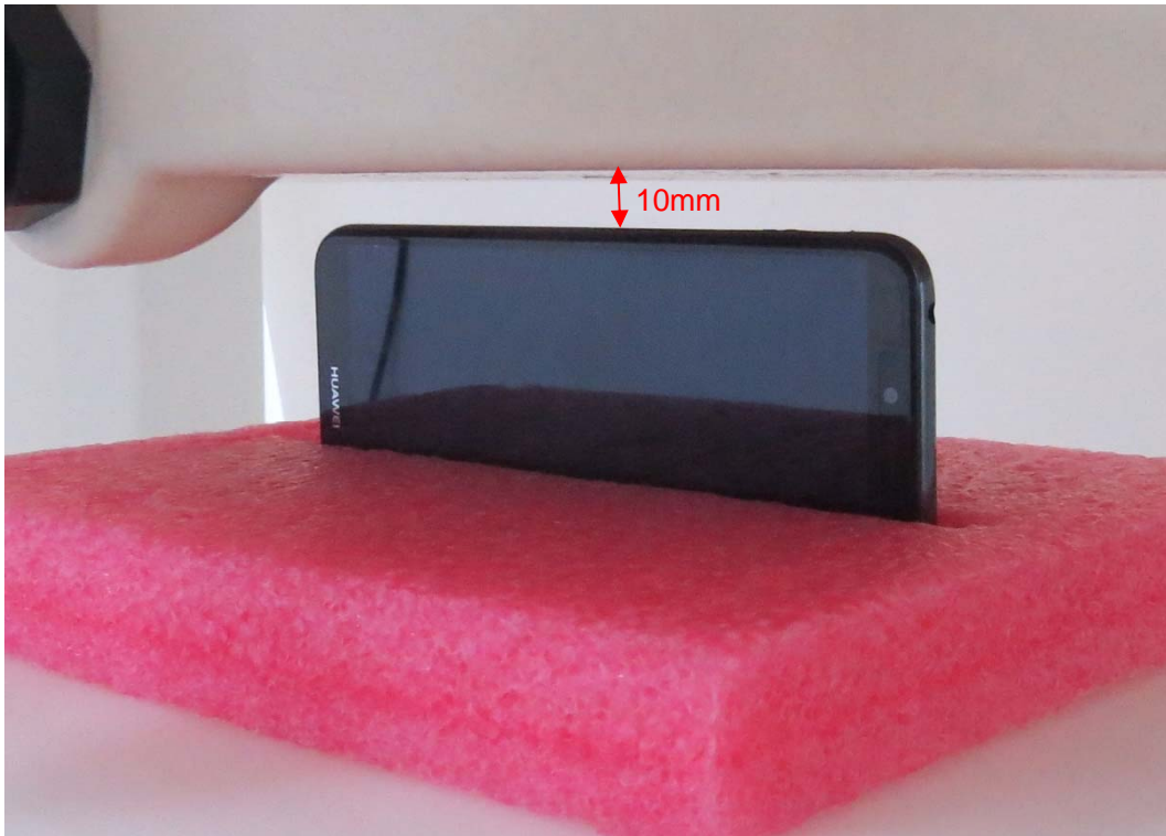
Picture 9: Left Side, the distance from handset to the bottom of the Phantom is 10mm (ATU-L11)
