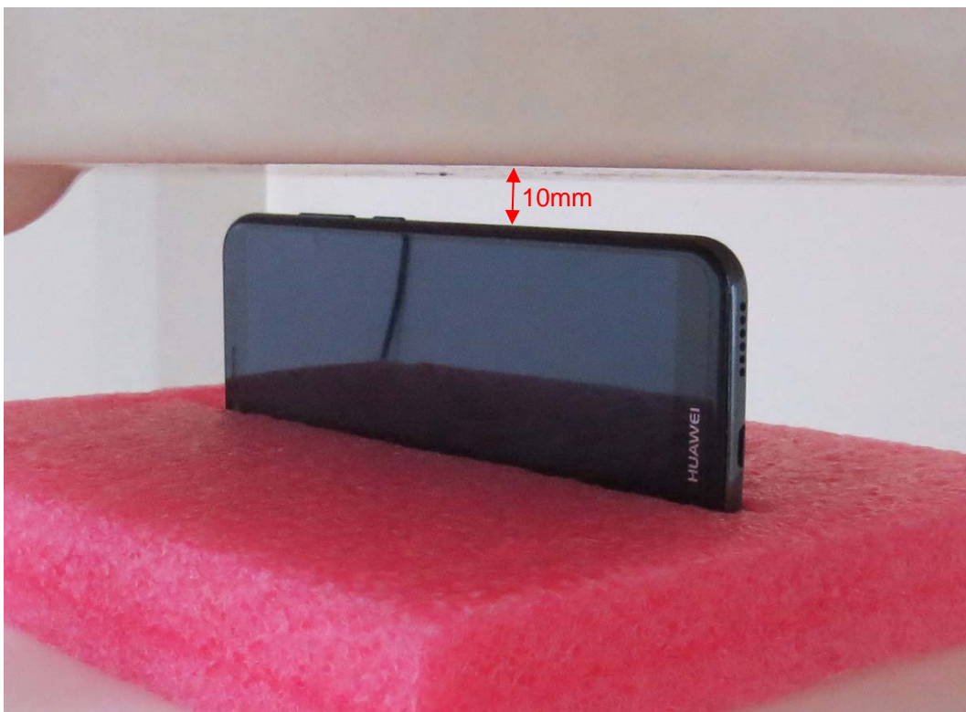
Picture 10: Right Side, the distance from handset to the bottom of the Phantom is 10mm (ATU-L11)
