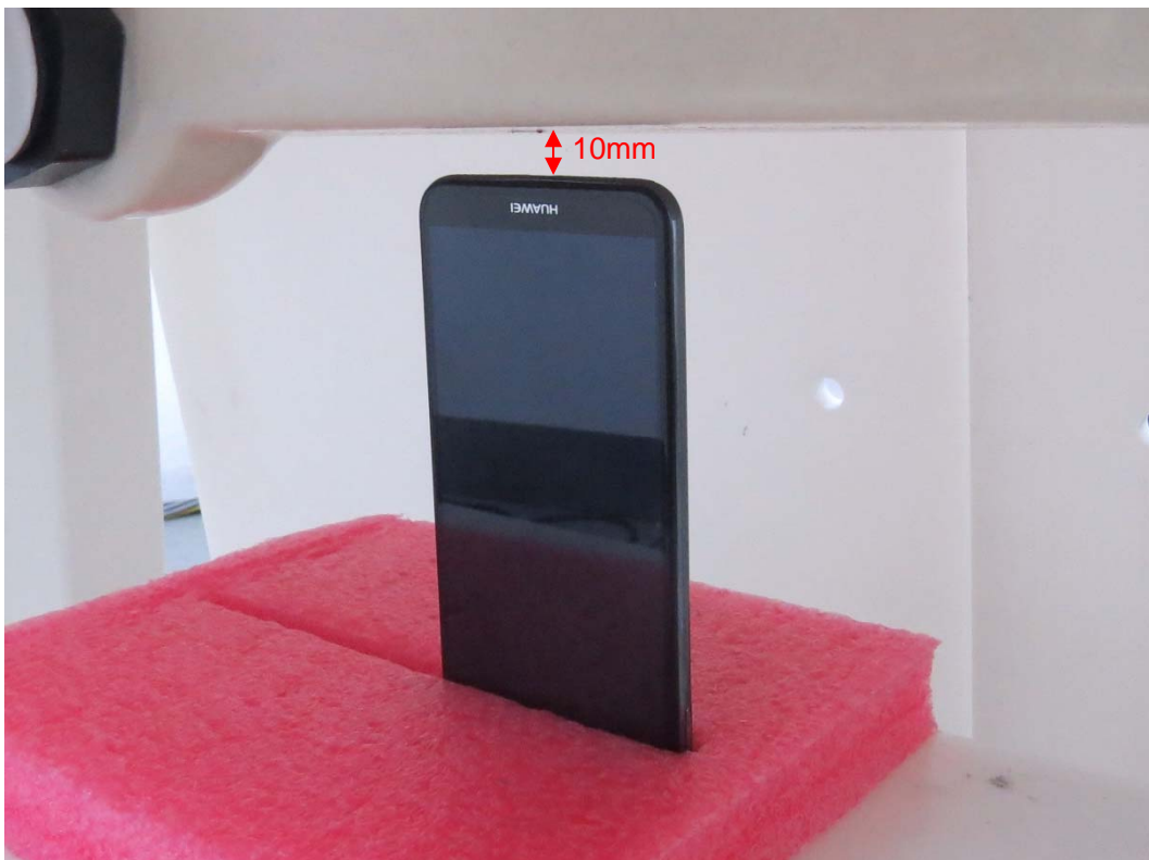
Picture 12: Bottom Side, the distance from handset to the bottom of the Phantom is 10mm (ATU-L11)
