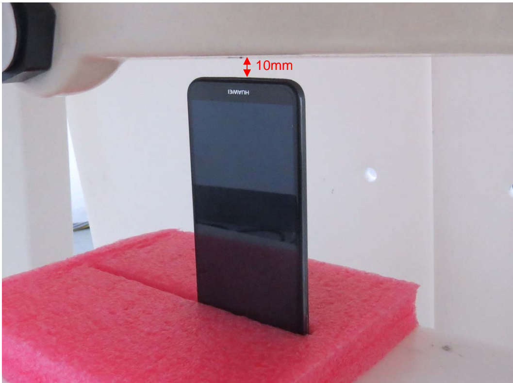
Picture 12: Bottom Side, the distance from handset to the bottom of the Phantom is 10mm
