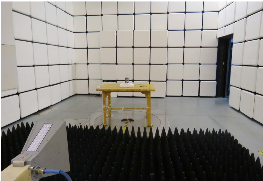
Picture 1: Radiated Spurious Emissions Test setup
