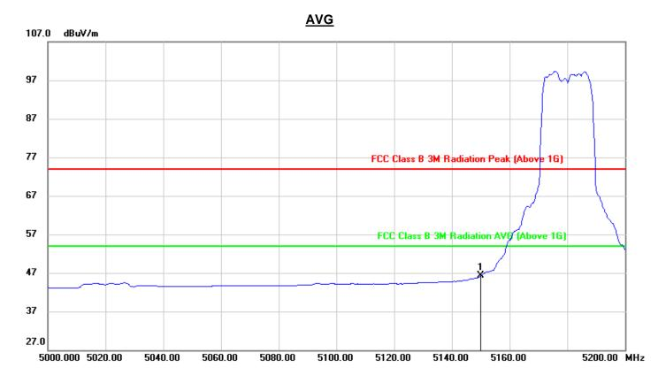
Frequency Reading Correct Margin Remark No. Result Limit (dBuV/m) dB/m (dBuV/m) (dBuV/m) (MHz) (dB) 5150.000 5.83 40.40 46.23 54.00 -7.77 AVG
