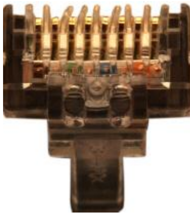
Figure 5-83 Skewed plastic separators
