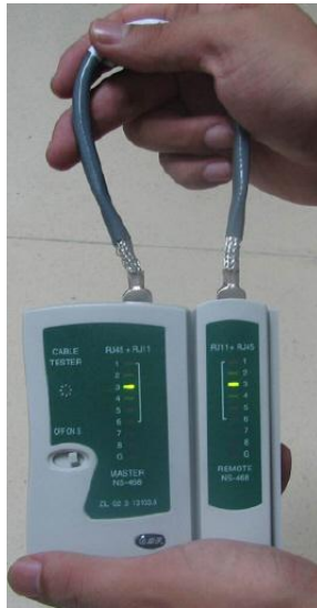
Figure 5-87 Checking the reliability
