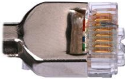
Figure 5-82 Dirt on a contact strip
