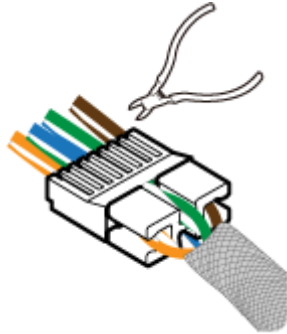
Figure 5-53 Neatly cutting edge cables
