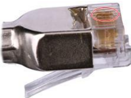
Figure 5-81 Unparallel contact strips of different heights
