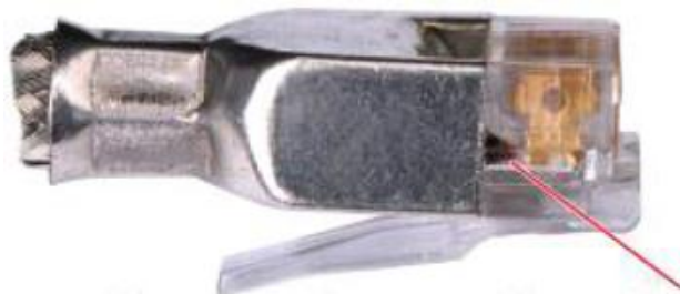
Figure 5-84 Wires not in good contact with the edge of the RJ45
