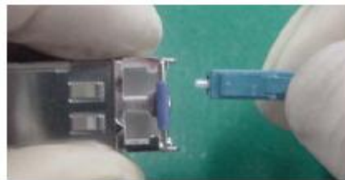
Figure 5-171 Using fibers to protect an optical module
