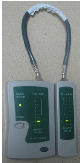
Figure 5-86 Testing the conduction and connections of wires
