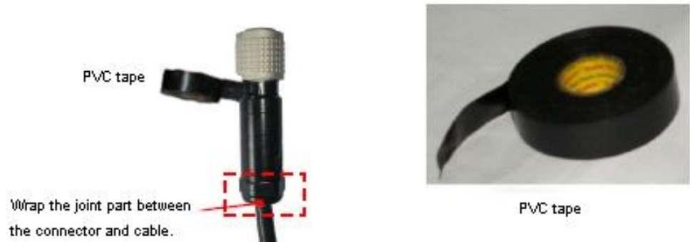
Figure 5-117 Wrapping the PVC tape
