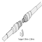
Figure 5-95 Installing the connector
