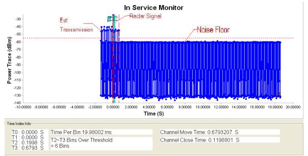
Note: T1 denotes the start of Channel Move Time upon the end of the last Radar burst.
