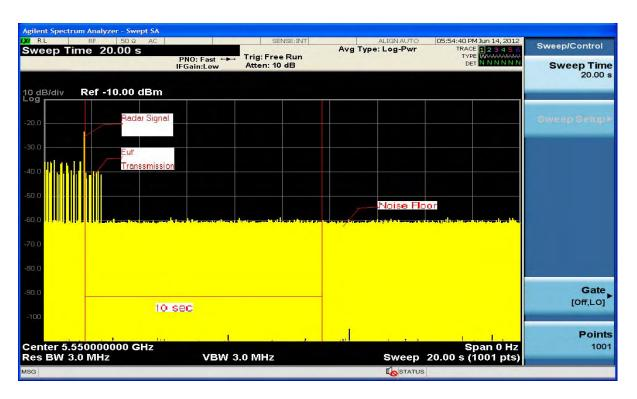
Note: An expanded plot for the device vacates the channel in the required 500ms
