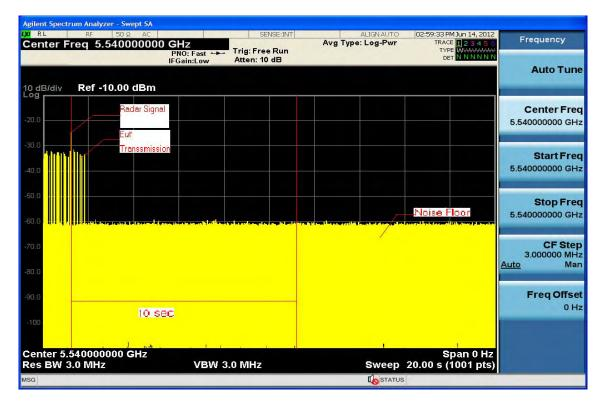
Note: An expanded plot for the device vacates the channel in the required 500ms
