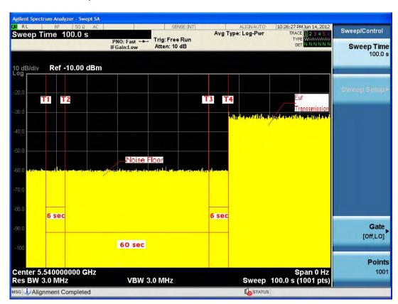
**Note:** T1 denotes the end of power-up time period is 7 second. T4 denotes the end of Channel Availability Check time is 67 second. Channel Availability Check time is equal to (T4 – T1) 60 seconds.
