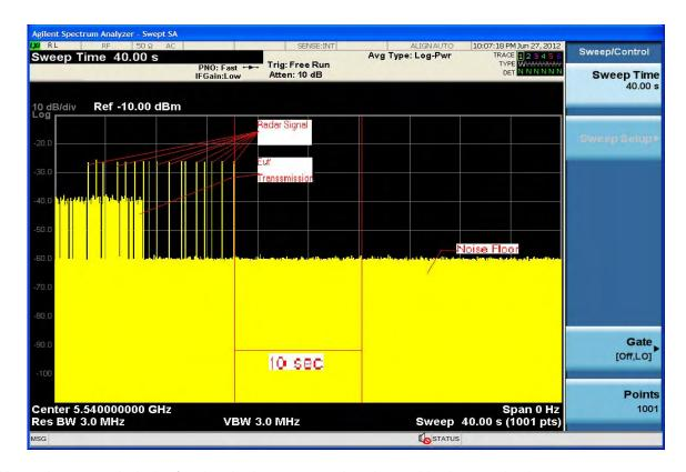
Note: An expanded plot for the device vacates the channel in the required 500ms
